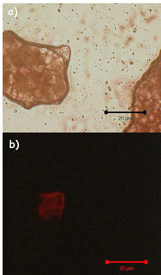
Figure 4.17. Light microscopy (a) and fluorescence microscopy (b) images of RuNH-M-ETS-10.
