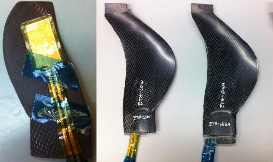
**Figure 1-7. Open rotor aircraft engine composite blades with piezoelectric elements [7]**
