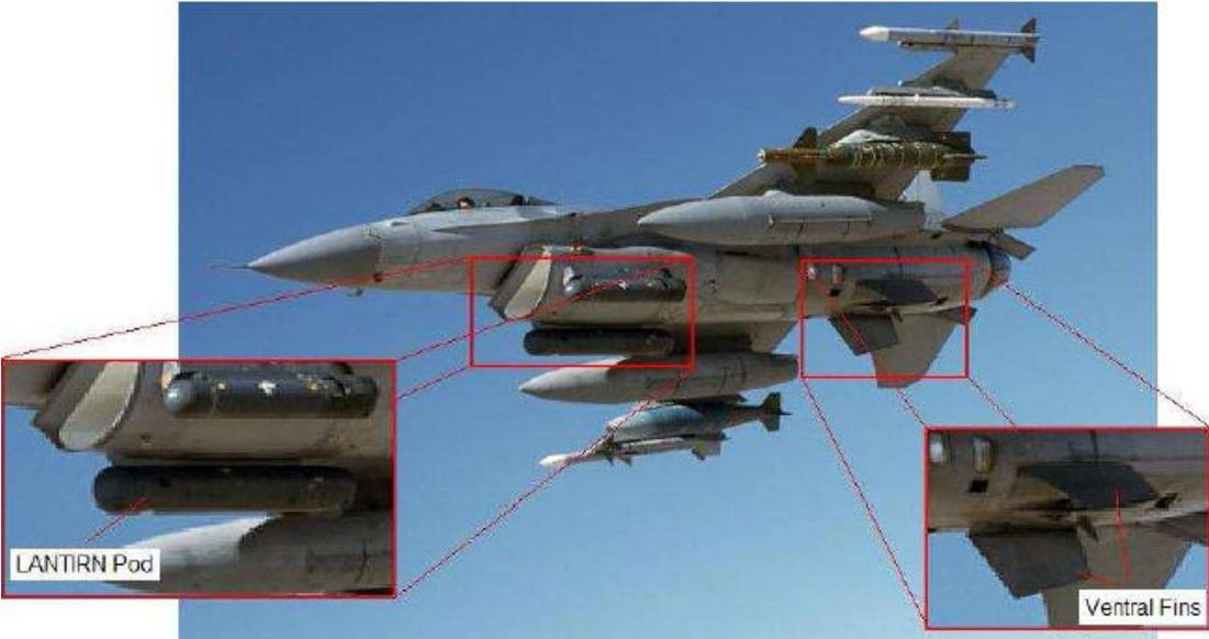
**Figure 1-1. LANTIRN pods and ventral fins of F-16 aircraft [9]**
