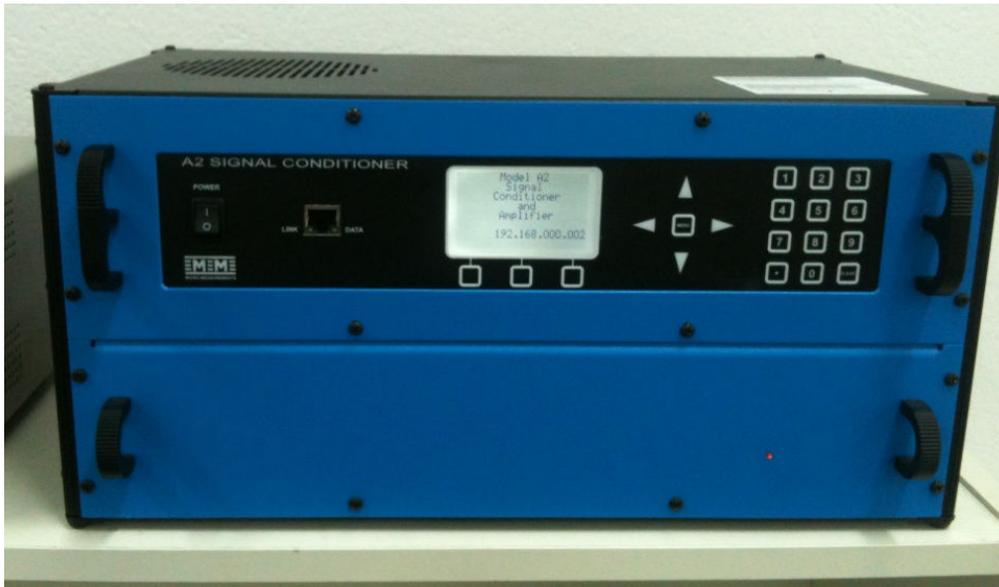
**Figure 3-37. Micro Measurement Model A2 Strain gage conditioning unit**
