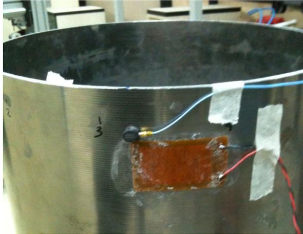
**Figure 4-28. Accelerometer placed at the corner of the piezoelectric actuator**
