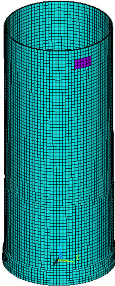
**Figure 4-4. Finite element mesh over the 3-D cylinder model**
