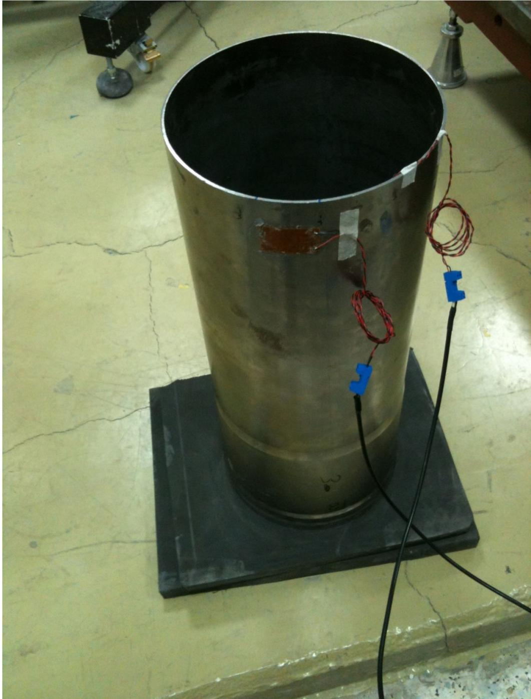
**Figure 4-26. Piezoelectric patch on the outer surface of the cylinder**
