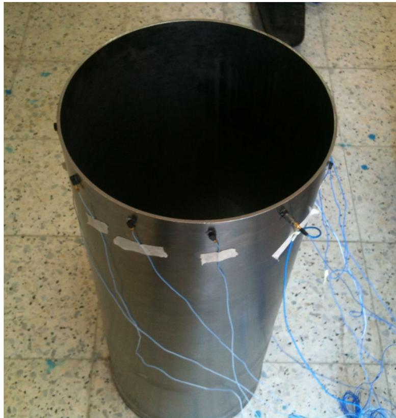
**Figure 4-38. Accelerometers placed on the cylinder for modal test**
