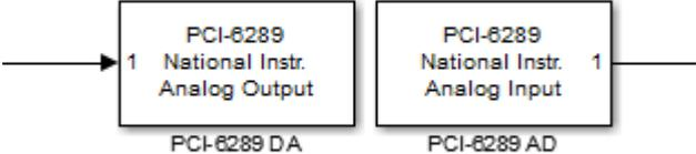
**Figure 3-39. Simulink blocks for NI PCI card**
