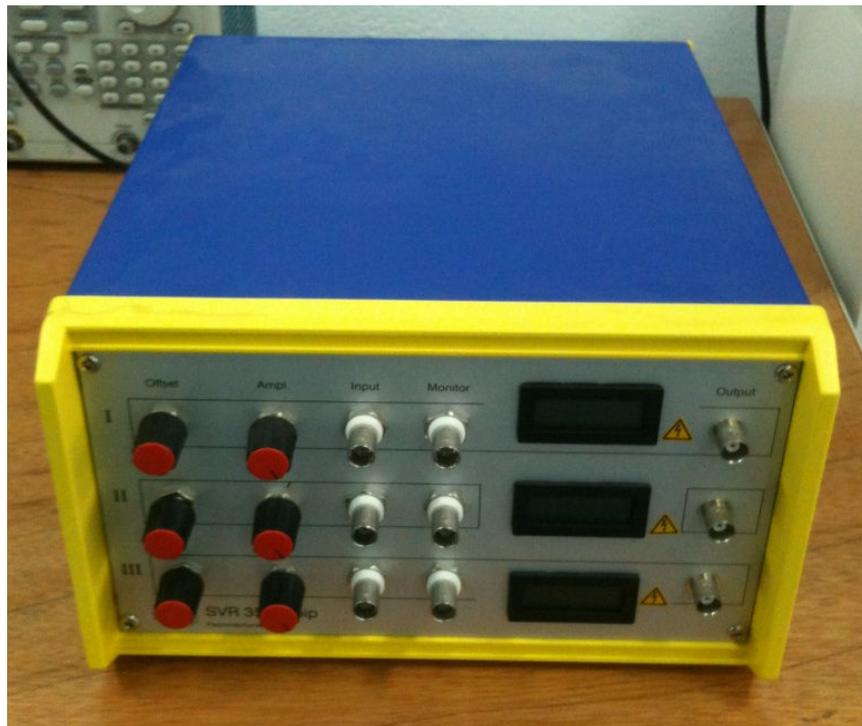
**Figure 3-38. APC SVR 350-bip piezoelectric voltage amplifier**
