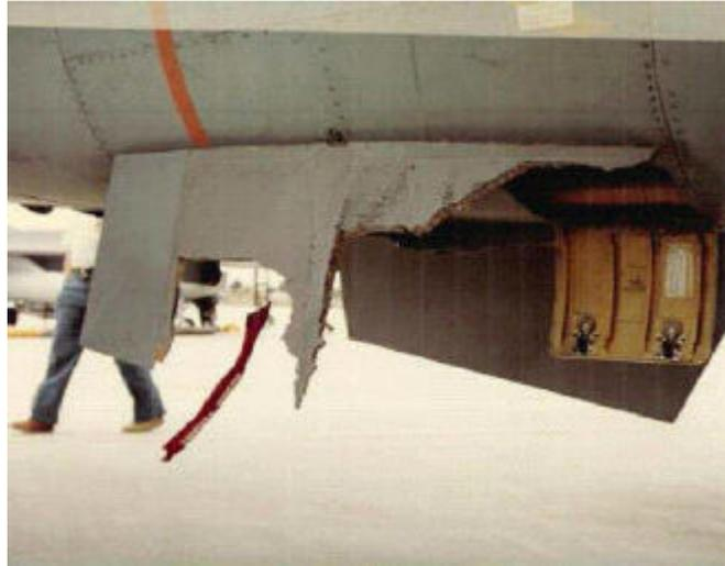
**Figure 1-2. Ventral fin failure [9]**
