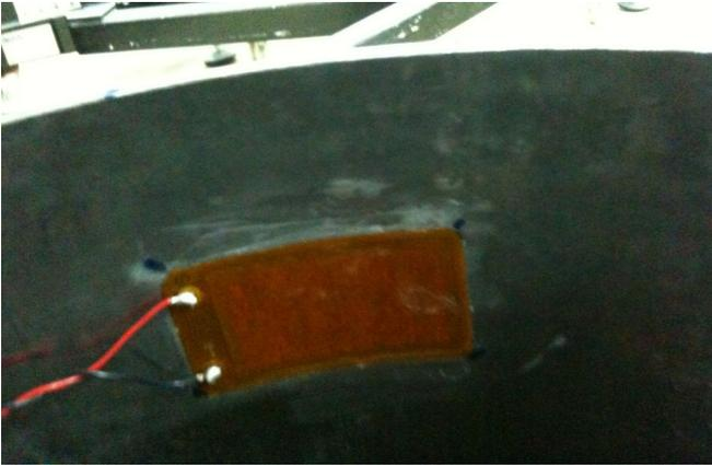
**Figure 4-27. Piezoelectric patch on the inner surface of the cylinder**
