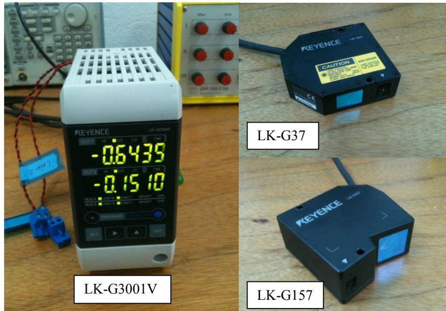
**Figure 3-36. Keyence laser displacement sensor and controller unit**
