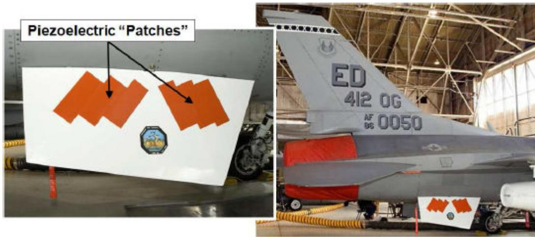
Figure 1-3. Test fin with piezoelectric patches [9]
