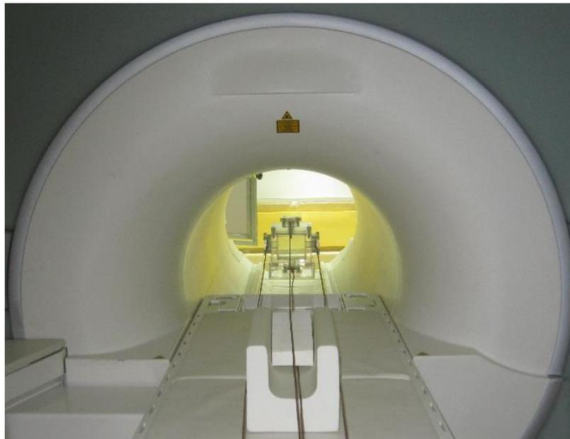
Figure 3.12: Illustration of the experimental phantom inside the MR magnet
