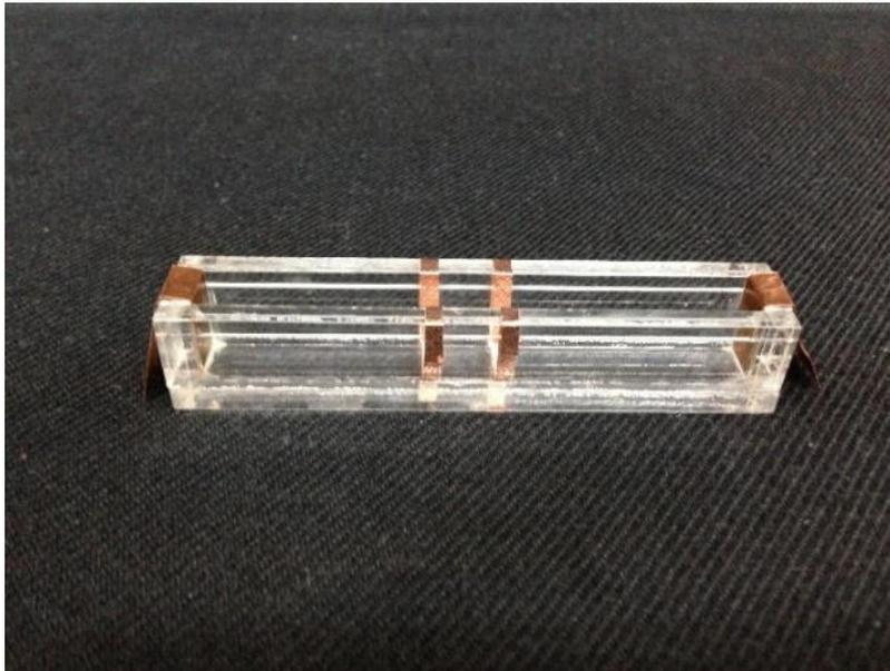
Figure 3.13: conductivity cell
