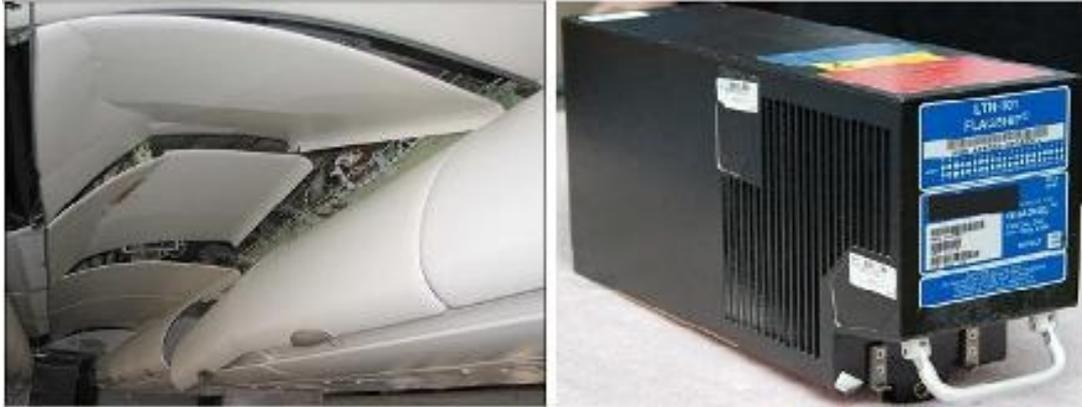
Figure 2.1: Damage of Qantas Flight(left), Air Data Inertial Reference Unit(right).
