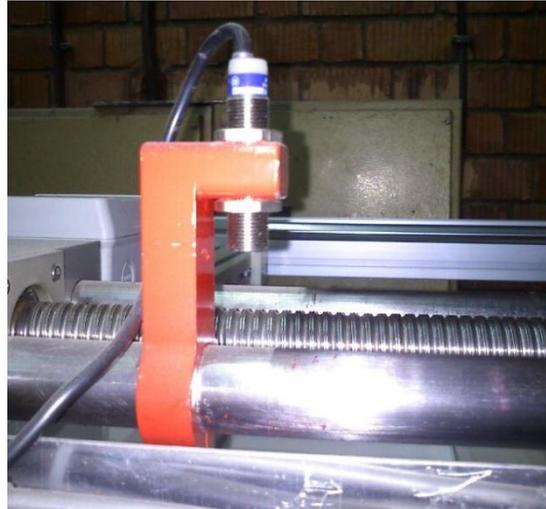
Figure G.4 Sensor of Traverse Mechanism
