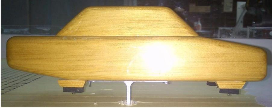
Figure 4.6 MIRA Model Attached to the Test Set-up
