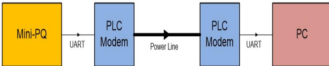
Figure 5.5: Block diagram for the minimum mode of the Mini-PQ.
