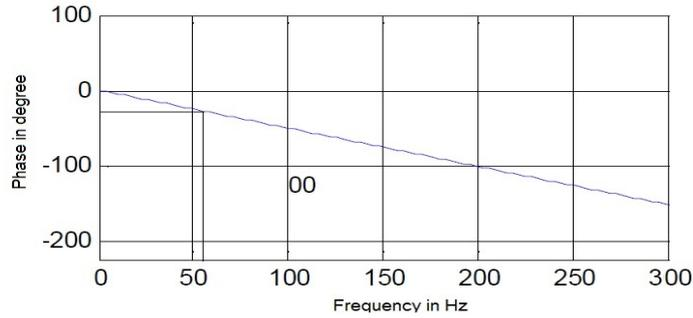
Figure 3.3: Phase response of the LP FIR filter
