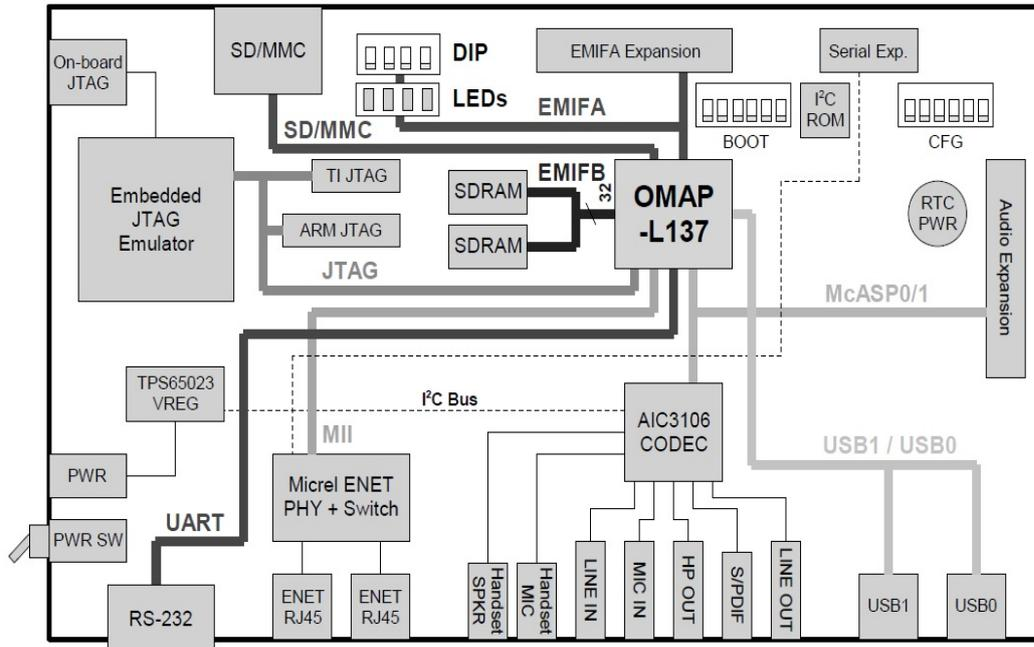
Figure 4.12: Block diagram of OMAP-L137 EVM [11]
