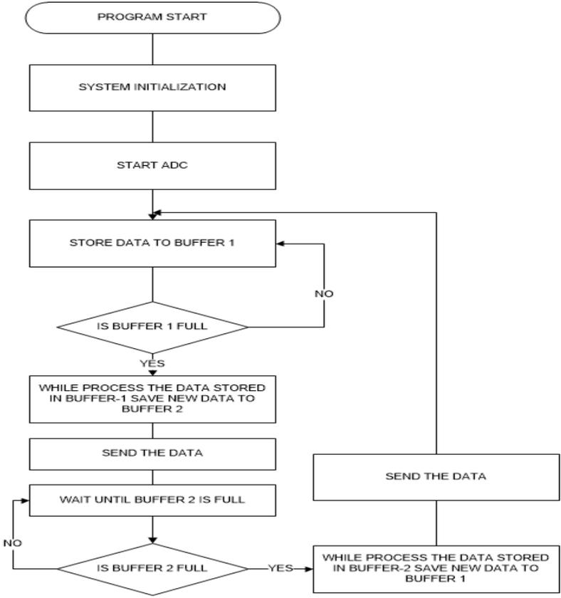
Figure 5.2: Block diagram of the DSP program.
