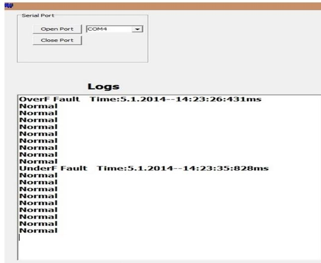
Figure 6.28: Under frequency error on the GUI.
