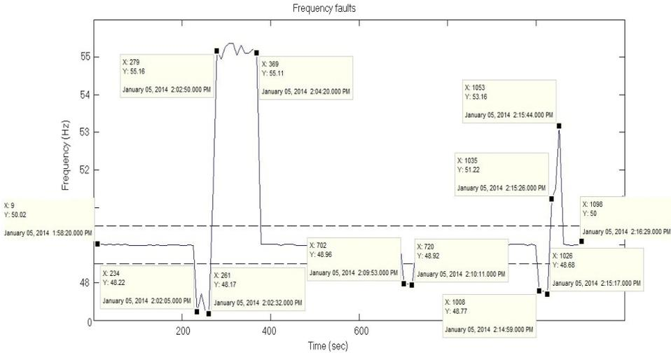
Figure 6.17: Under and over frequency faults.
