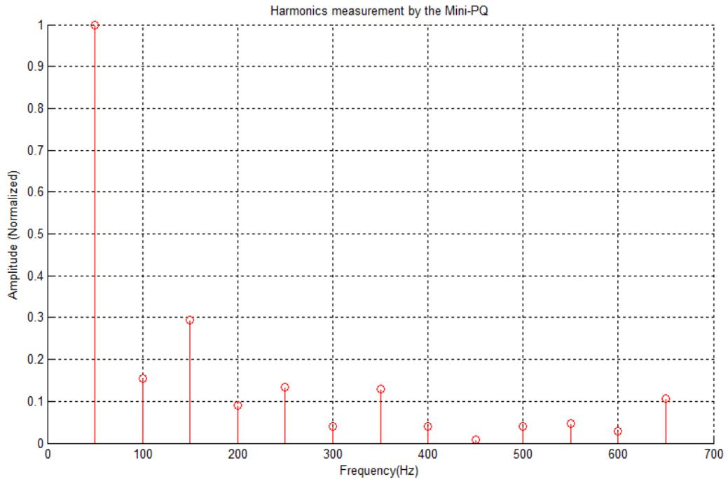
Figure 6.23: Harmonics measurement of the Mini-PQ.
