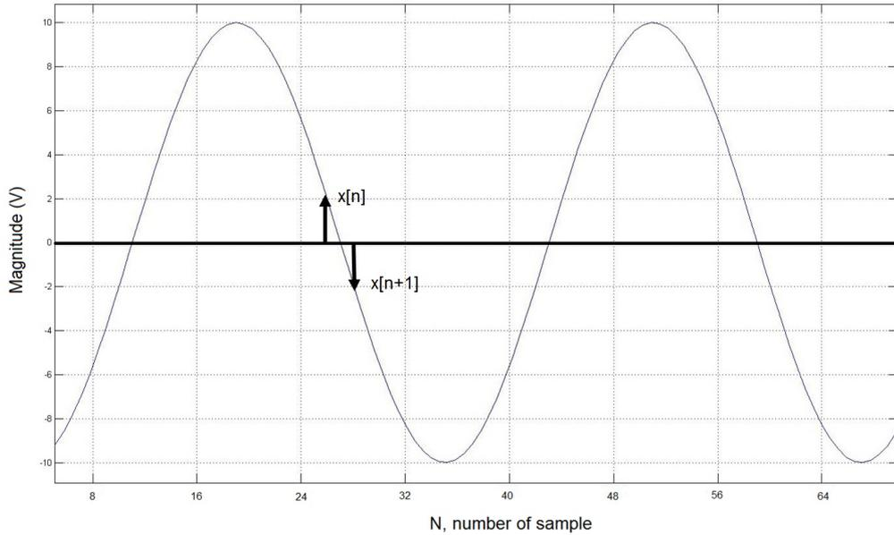
Figure 3.4: An example voltage signal for detecting zero crossing
