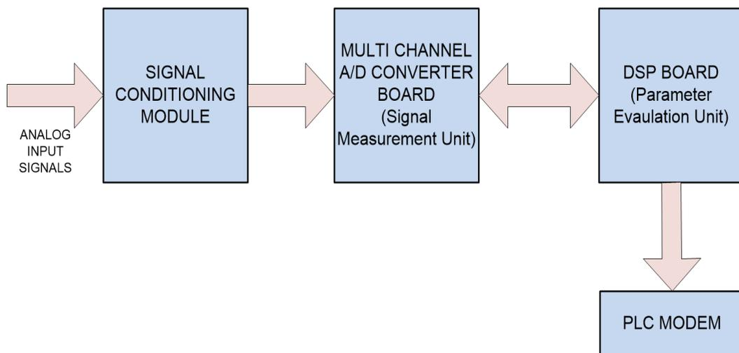
Figure 2.11: Simplified Measurement Setup of the Mini-PQ
