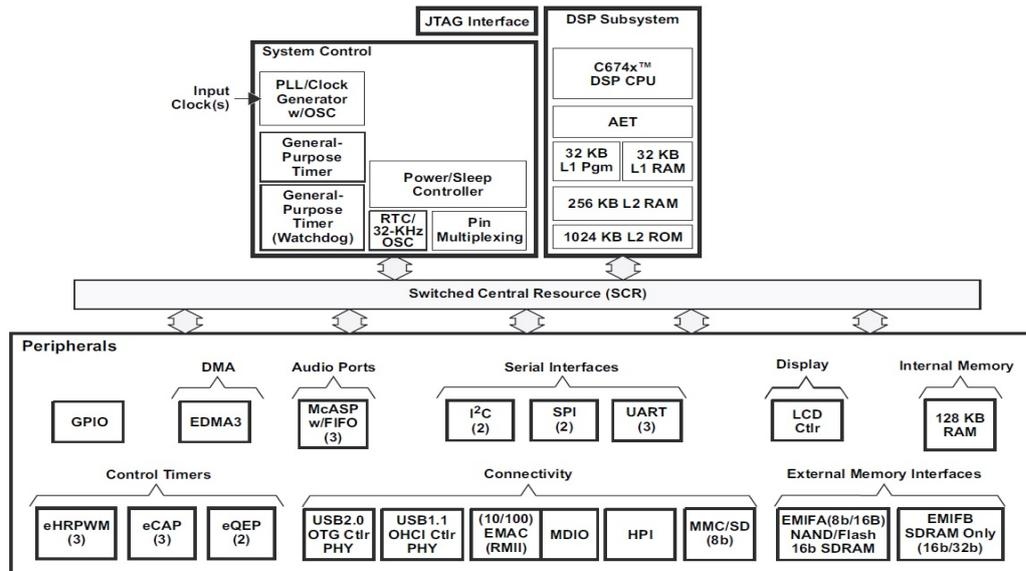
Figure 4.11: Functional block diagram of TMS320C6747 [10]
