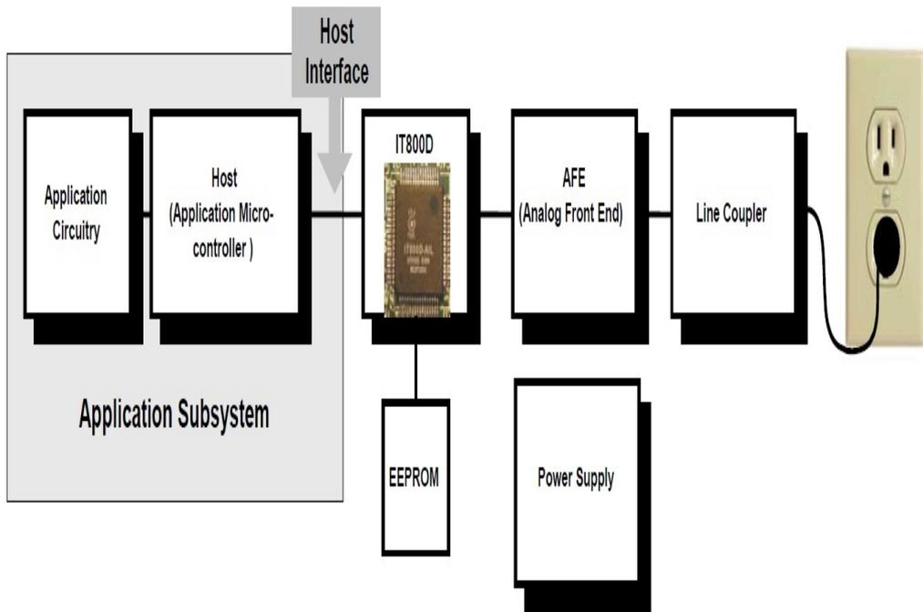
Figure 4.18: The PLC modem general scheme based on YITRAN IT800 [13]
