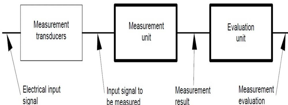
Figure 2.8: Measurement Chain [5]
