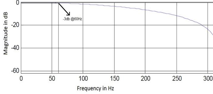
Figure 3.2: Frequency response of the LP FIR filter
