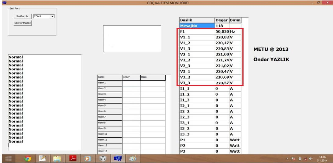
Figure 6.4: The Mini-PQ measurement for 220 Vrms output
