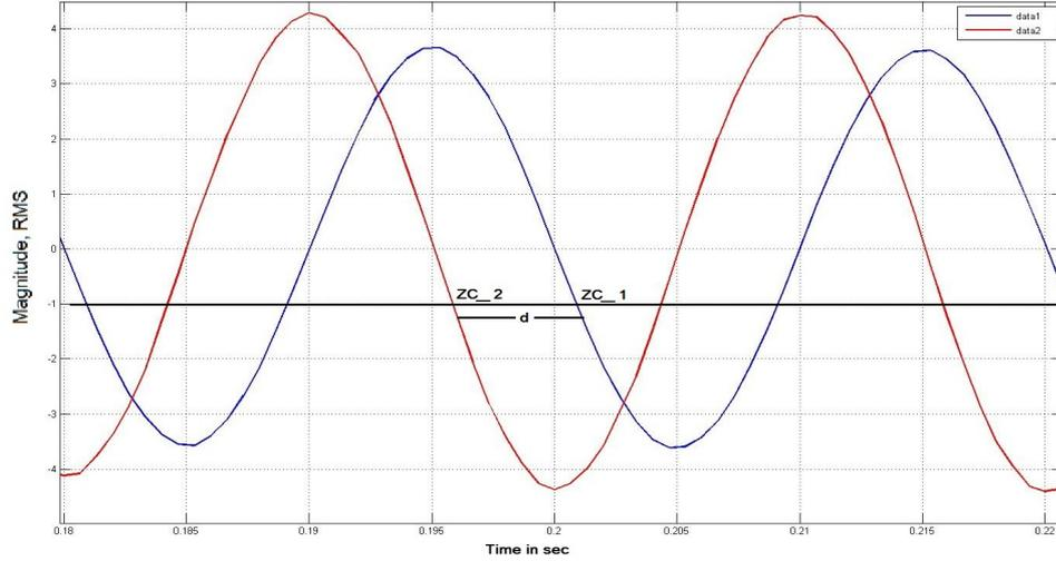
Figure 3.9: Voltage and current waveform which are out of phase
