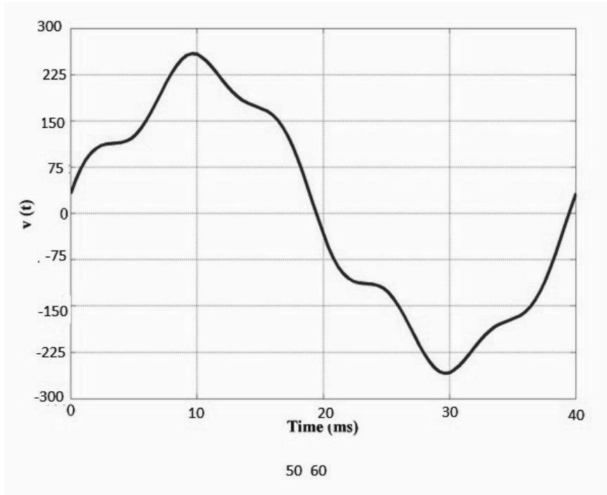
Figure 2.7: A Typical Distorted Waveform
