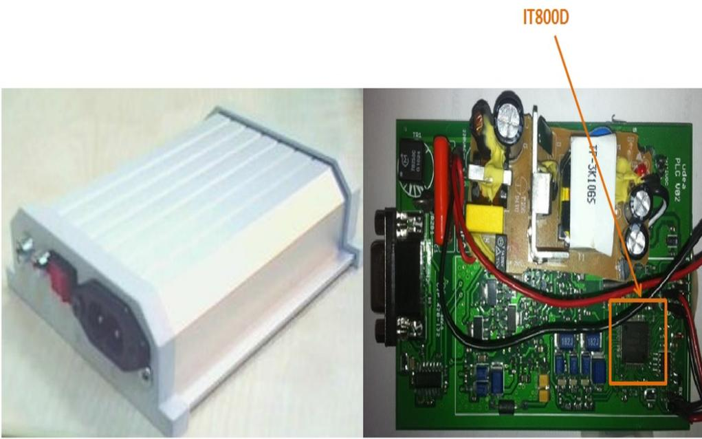
Figure 4.19: The PLC modem outside (left) and inside (right) view
