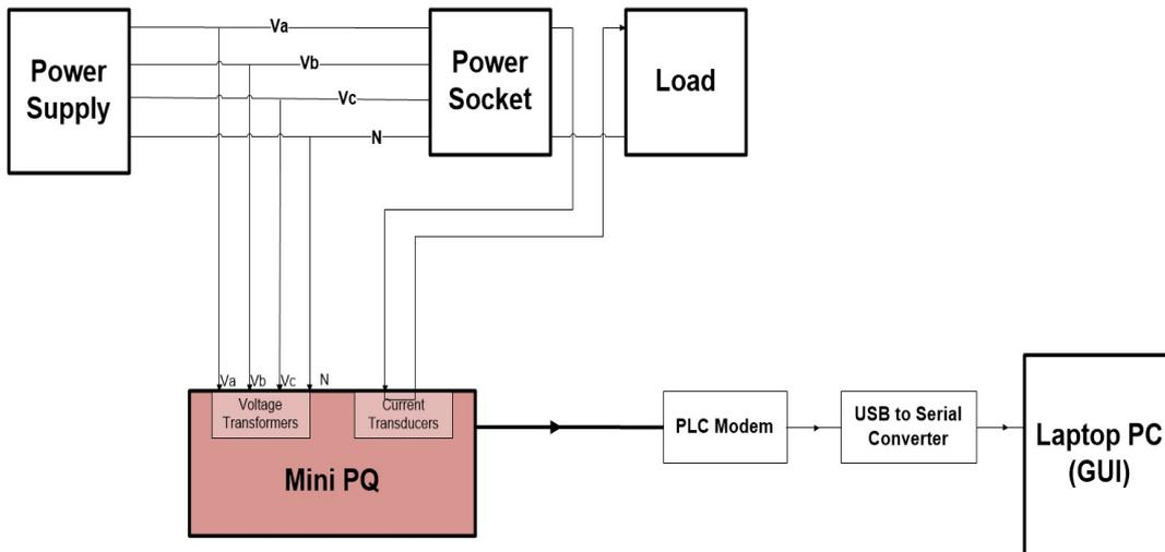
Figure 6.24: Block diagram for minimum mode field measurement..
