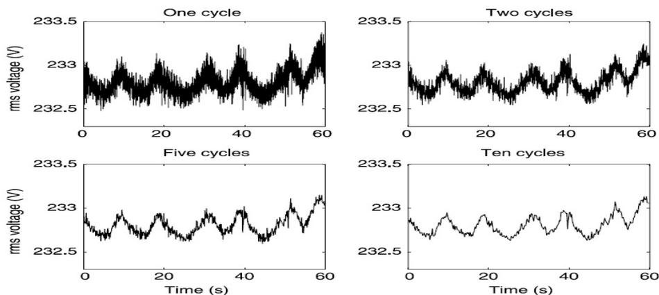
Figure 3.7: Effect of window length on RMS voltage versus time [4]
