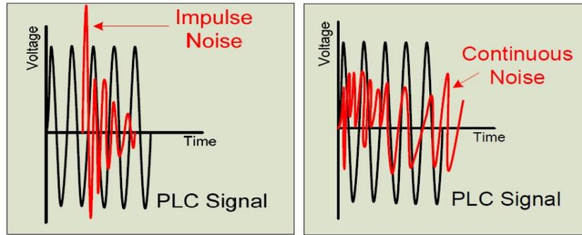
Figure 4.15: Impulse and continuous noise types on the power line [12]
