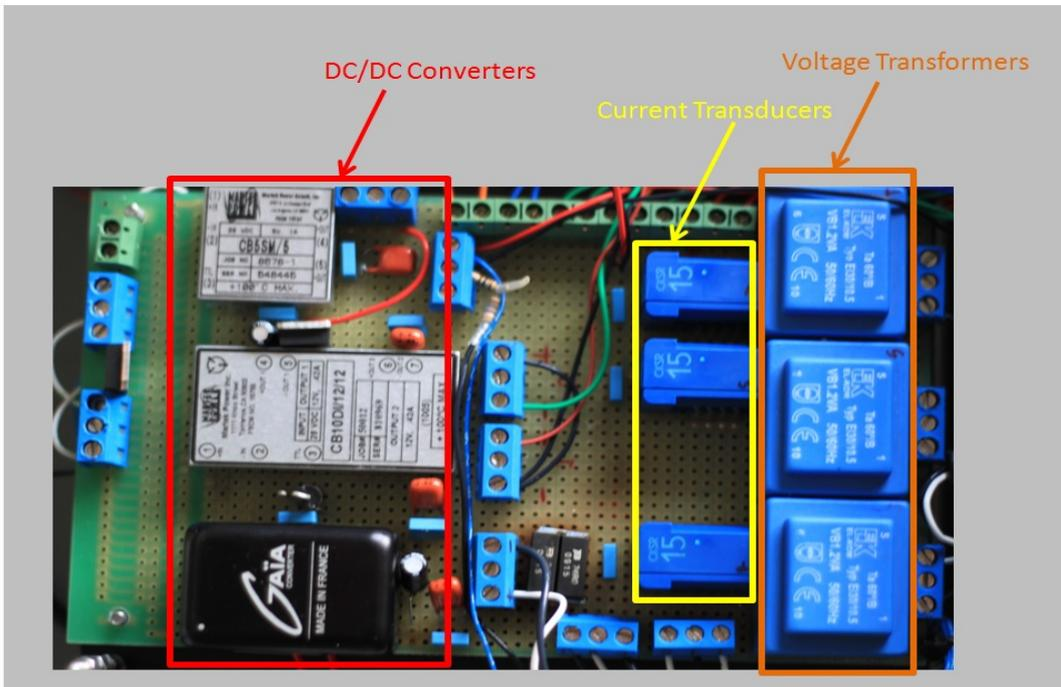
Figure 4.5: Signal Conditioning Card
