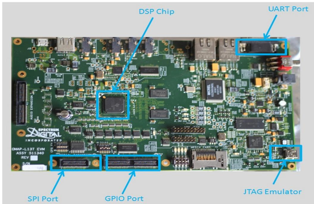
Figure 4.13: Picture of the digital signal processor unit
