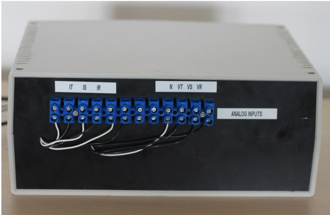
Figure 4.21: Analog input ports of the Mini-PQ
