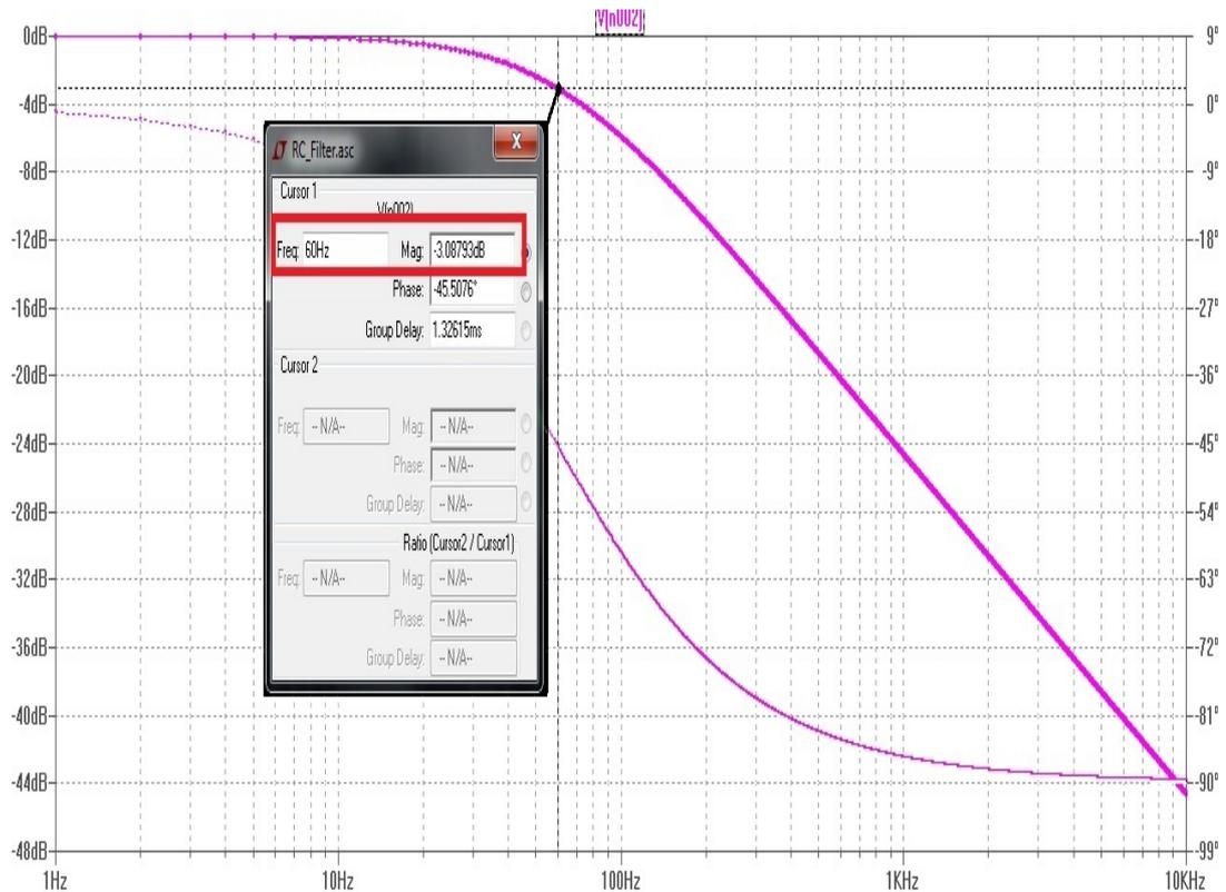
Figure 4.3: Frequency response of RC low pass filter
