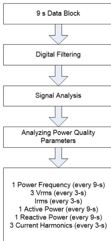
Figure 3.1: General flow diagram of data processing
