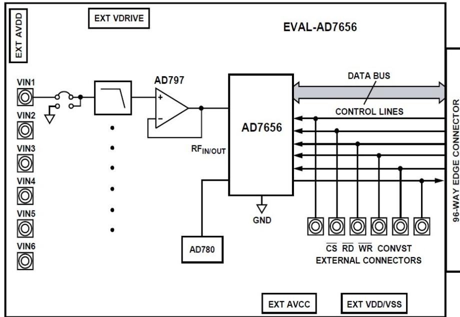
Figure 4.7: Functional block diagram of EVAL-AD7656 [8]
