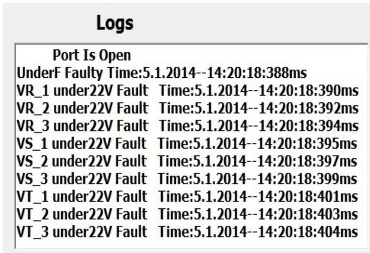
Figure 5.7: Logs window of the GUI.
