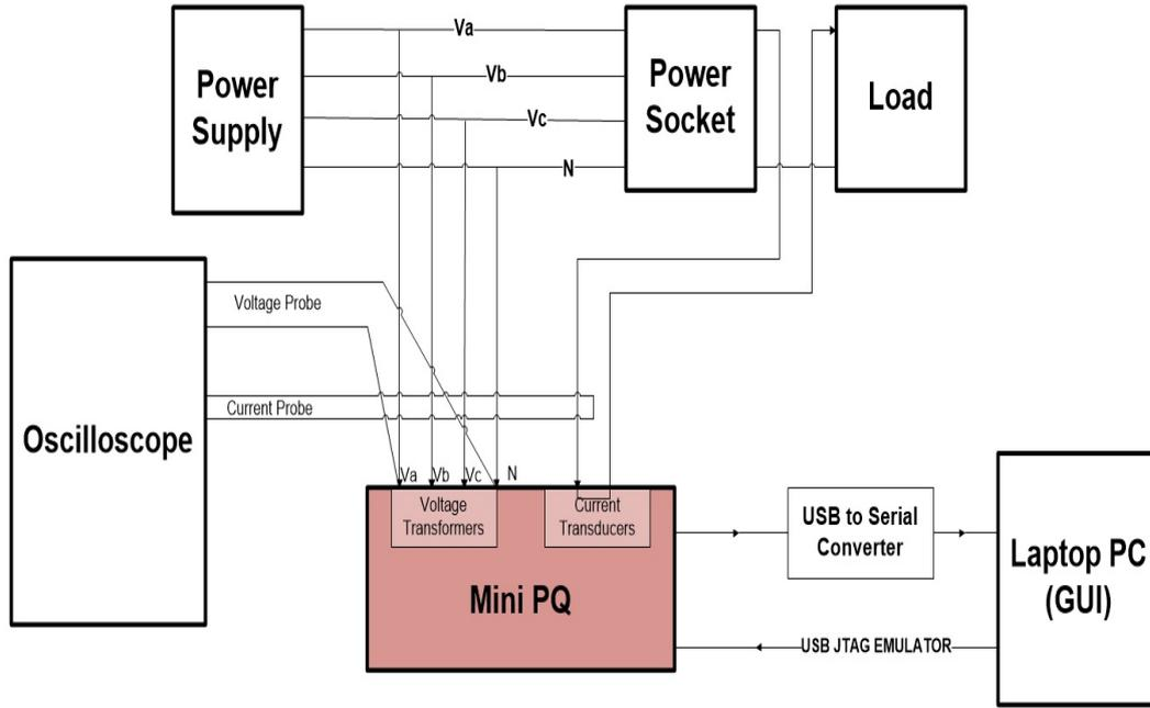
Figure 6.1: General block diagram of the test setup.
