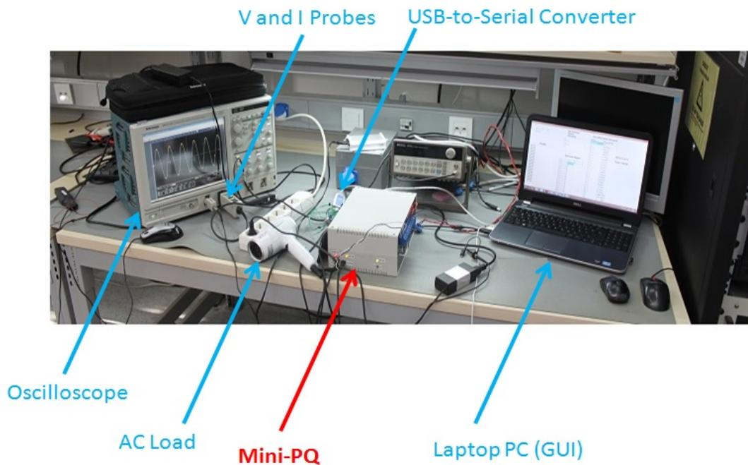
Figure 6.2: Picture of the measurement setup
