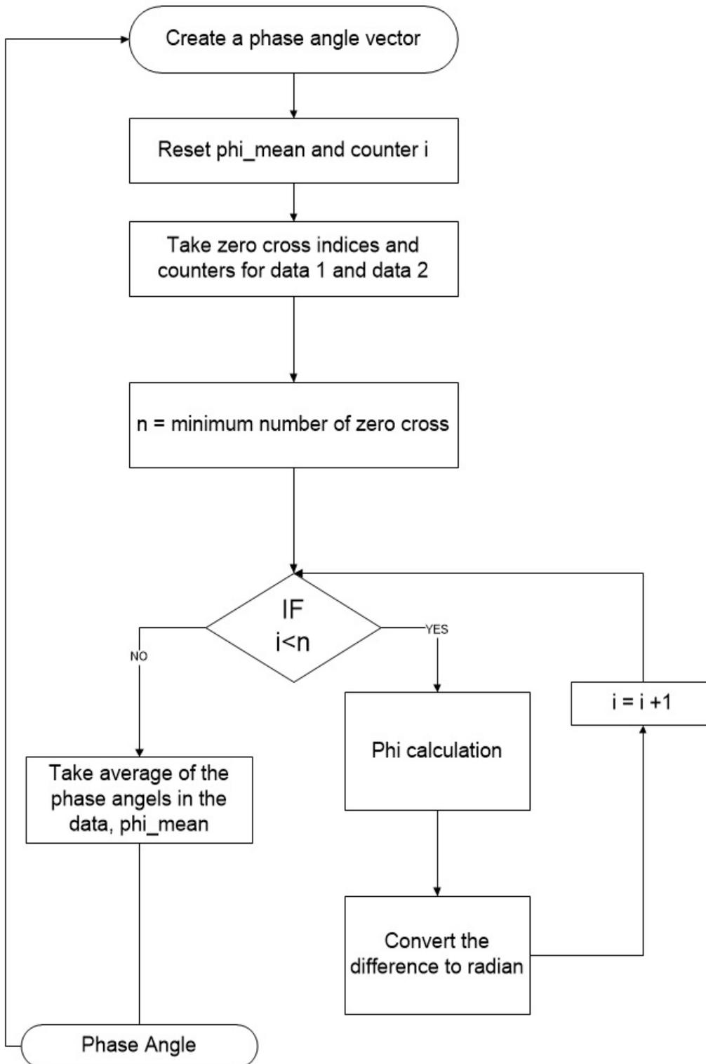
Figure 3.10: Flow chart for power calculation algorithm
