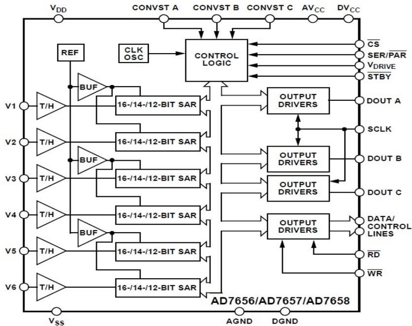
Figure 4.6: Functional block diagram of AD7656 REF
