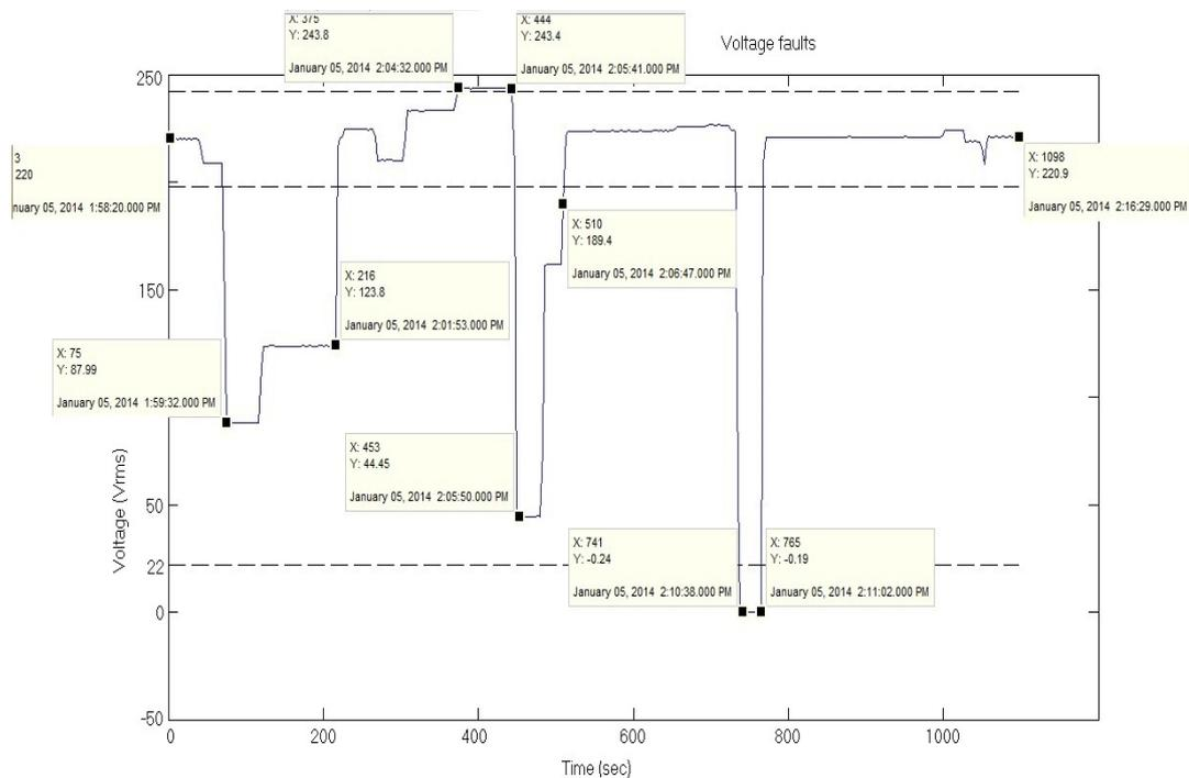
Figure 6.20: Voltage faults captured by the Mini-PQ.
