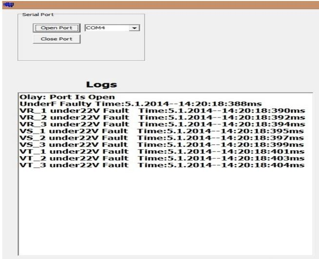
Figure 6.26: Voltage magnitude and interruption messages on the GUI.
