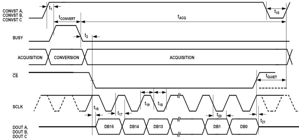
Figure 4.9: AD7656 Serial read operation [9]
