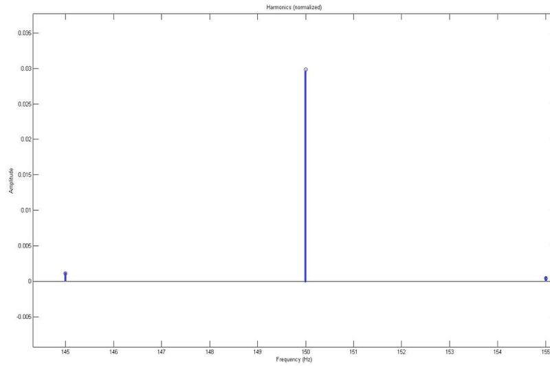
Figure 3.12: Spectral Leakage
