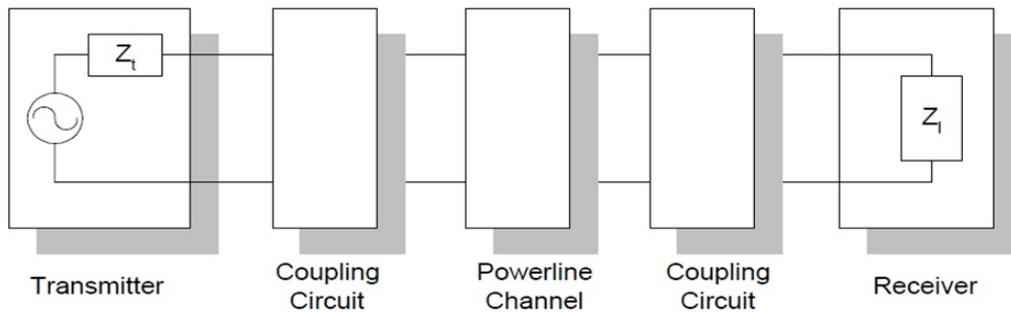
Figure 4.14: Block diagram of a powerline communication system
