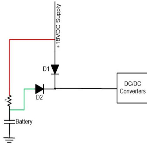
Figure 4.4: ORing and battery charging circuit
