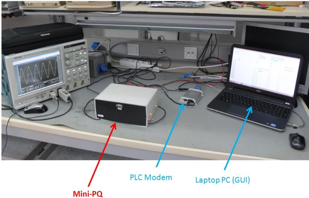
Figure 6.25: Picture of the setup for the minimum mode.
