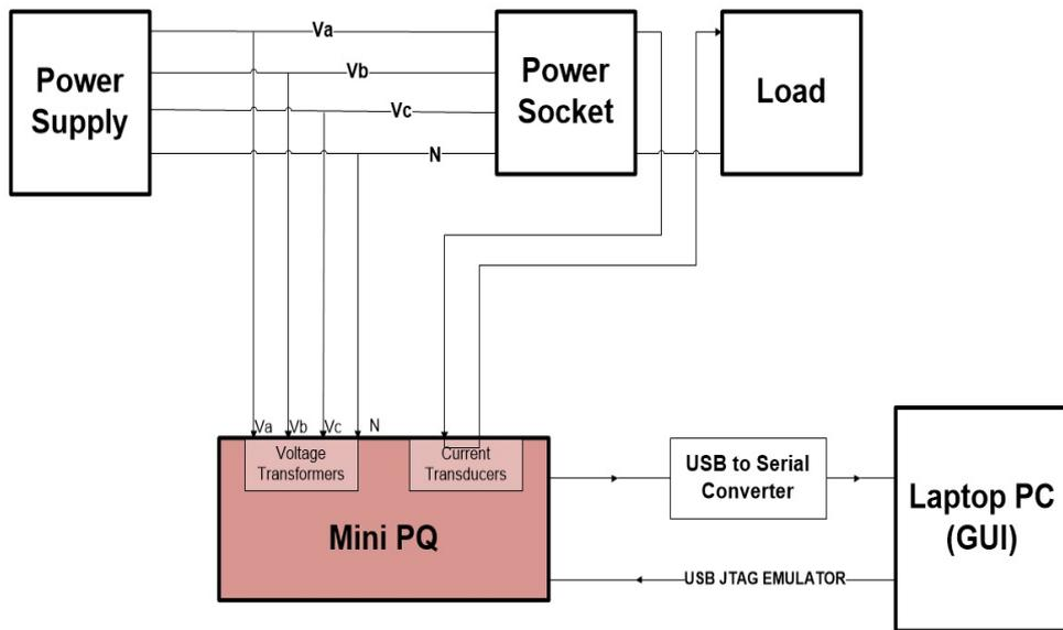
Figure 6.14: Block diagram for maximum mode field measurement.
