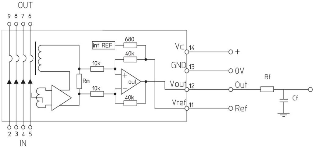
Figure 4.2: Current transducer functional block diagram [7]
