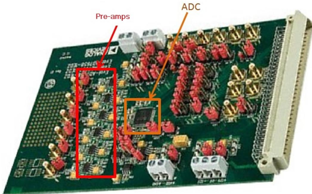
Figure 4.10: Analog to digital conversion unit
