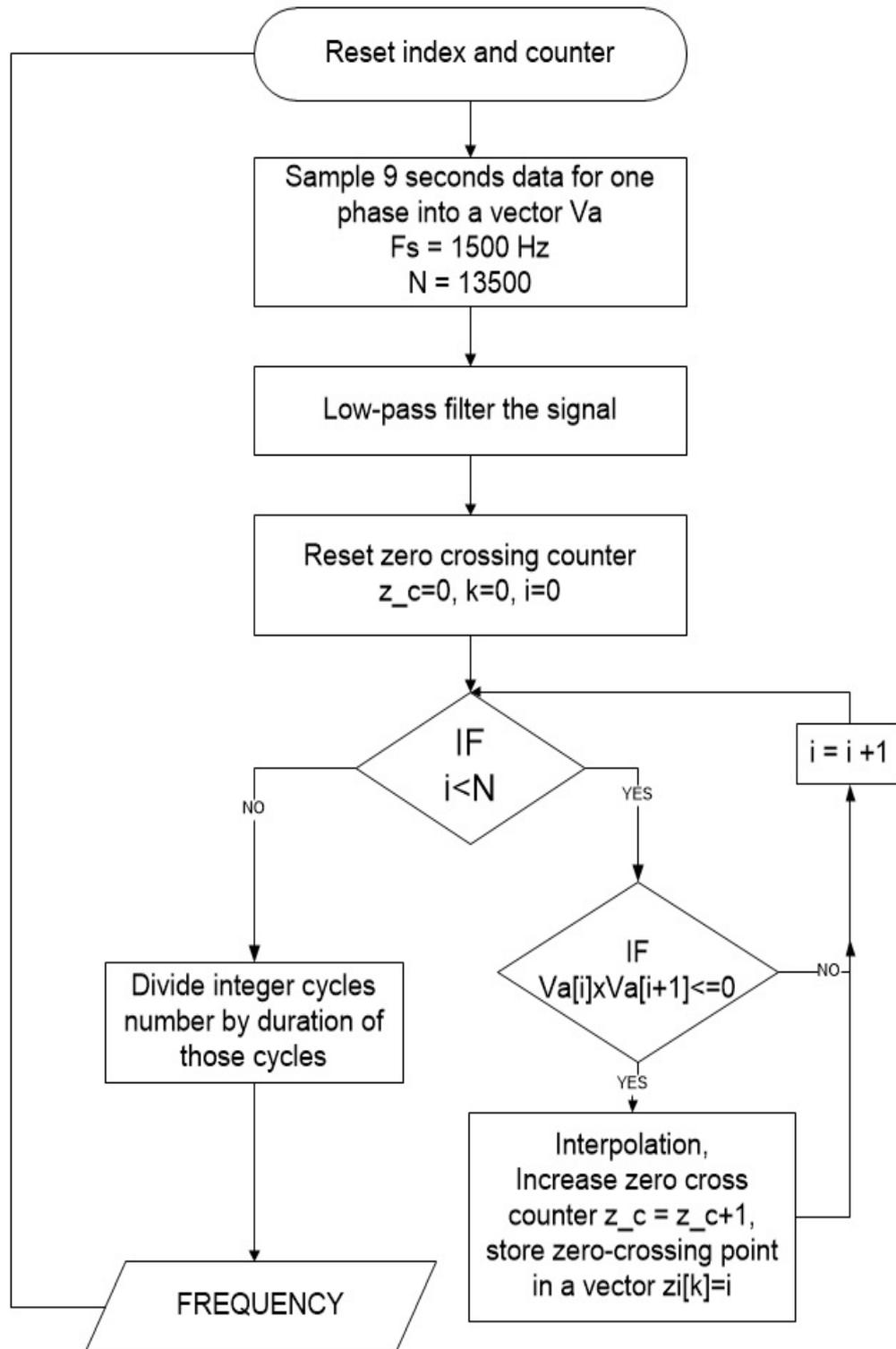
Figure 3.6: Frequency algorithm flow chart
