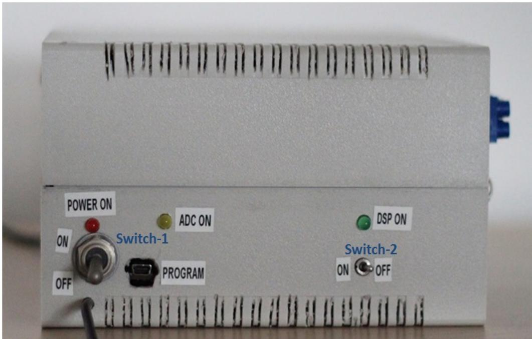
Figure 4.22: The Mini-PQ's switches and LEDs
