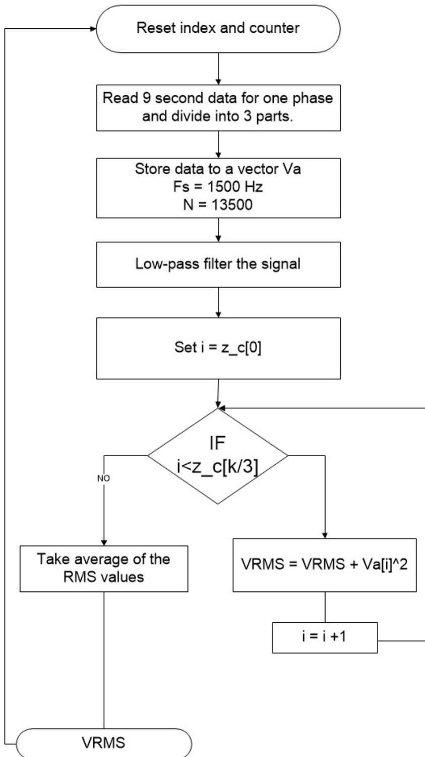
Figure 3.8: Flow chart for RMS calculation algorithm
