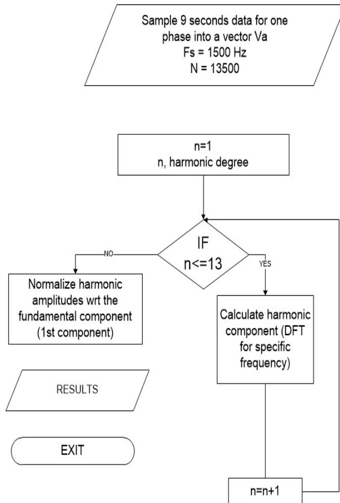
Figure 3.13: Flow chart for harmonics calculation algorithm
