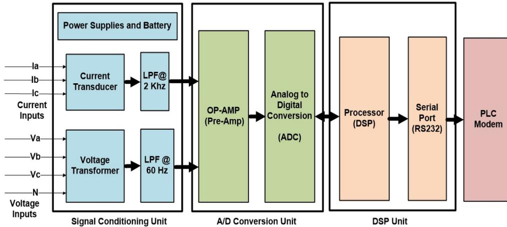
Figure 4.1: Simplified hardware block diagram of the Mini-PQ
