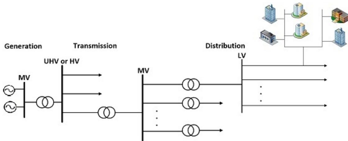
Figure 2.1: Electrical Grid
