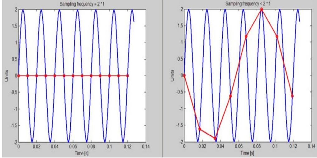
Figure 3.11: Illustration of the phenomenon of frequency aliasing [6]
