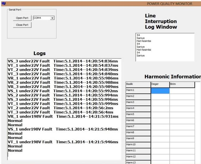
Figure 6.27: Normal frequency and under voltage fault messages on the GUI.
