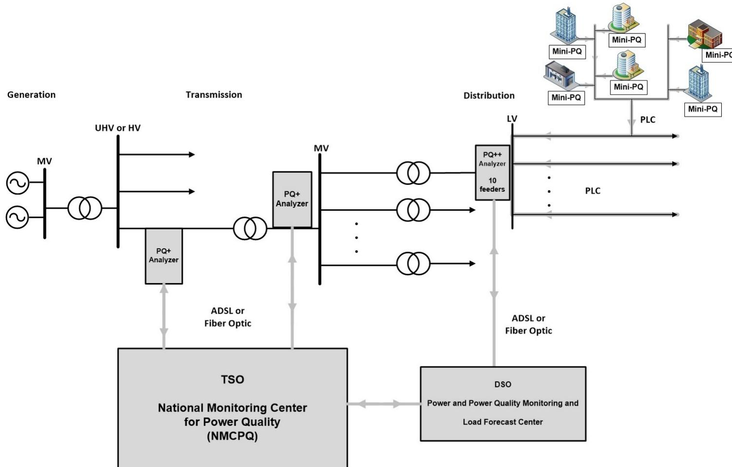
Figure 2.10: Conceptual illustration for the operation of the monitoring and control center together with multiple Mini-PQs and possible other monitoring and control centers. The gray lines indicate communication network between the monitors. The Mini-PQs use power line as the communication medium. TSO:Transmission System Operator, DSO:Distribution System Operator
