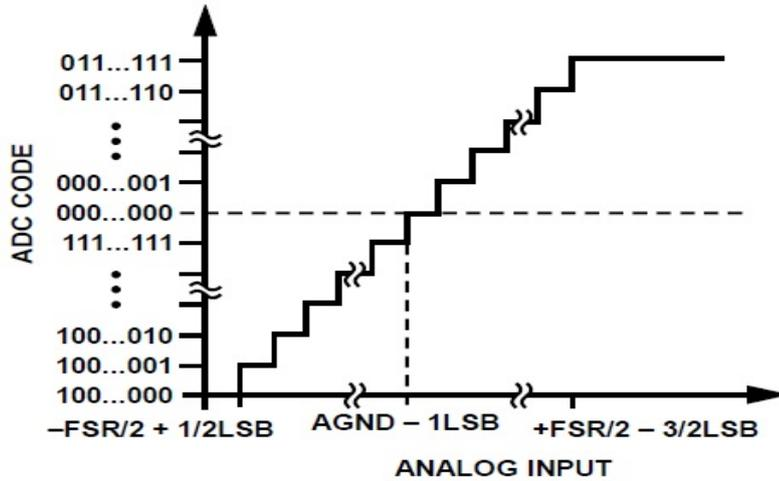
Figure 4.8: AD7656 Ideal transfer characteristic [9]
