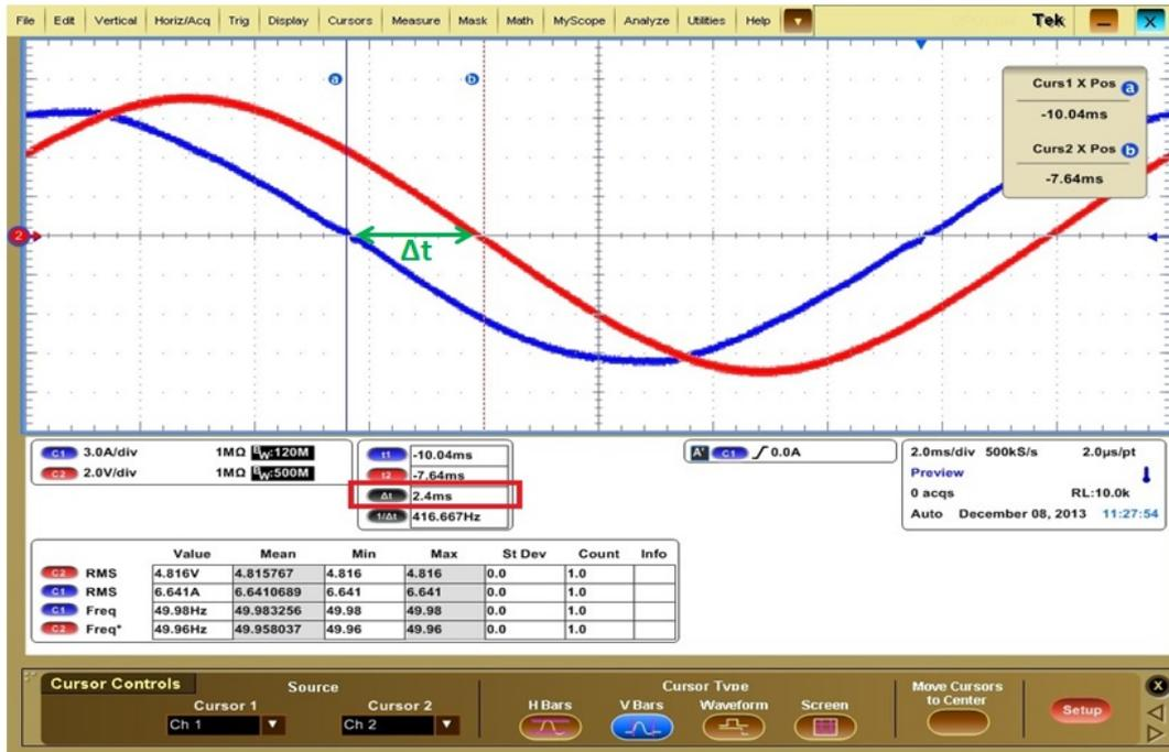
Figure 6.7: Time difference between the voltage and the current obtained by the oscilloscope.
