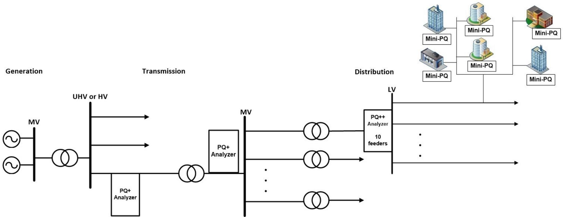
Figure 2.9: Conceptual illustration of the installed PQ monitoring devices in the Turkish electrical grid with multiple Mini-PQs
