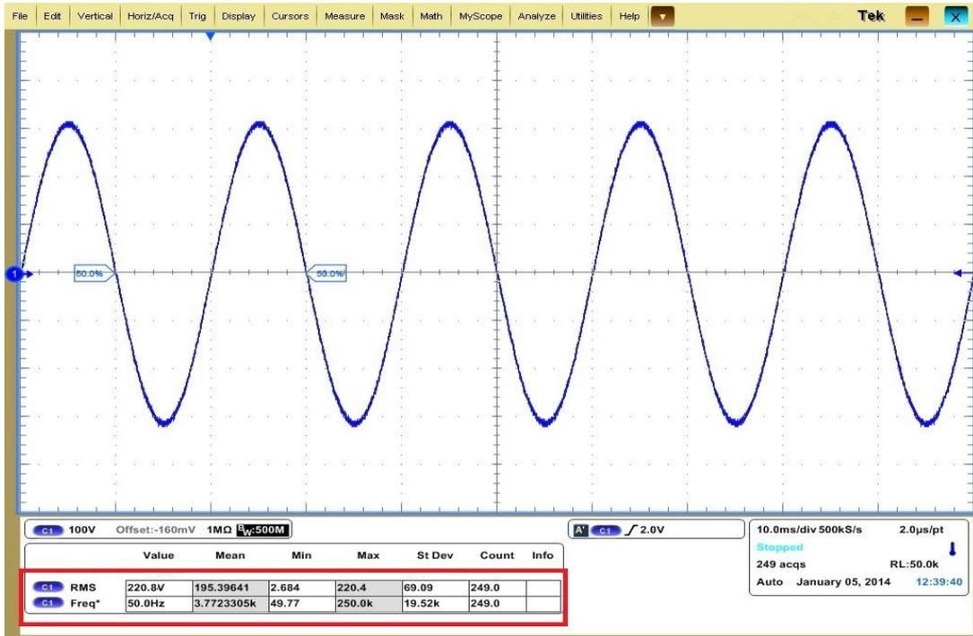
Figure 6.3: The oscilloscope measurement for 220 Vrms output
