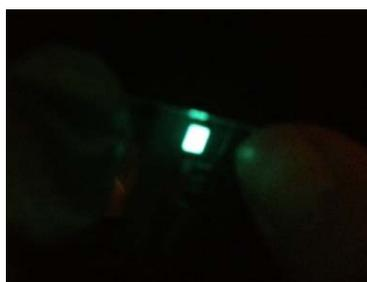
**Figure 71.** OLED device 6 using TPPE as an emitter
