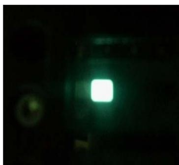
**Figure 76.** OLED device using TBIMPE as an emitter
