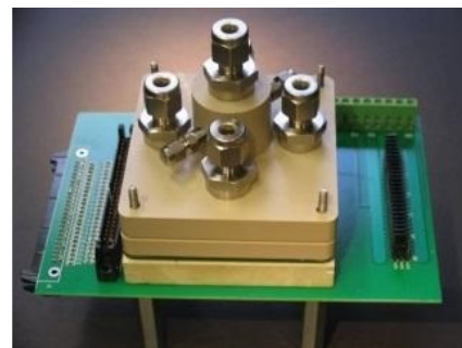
Figure 1.13: Fluid flow in jet impingement (left) Jet cooling module on PCB (right)
