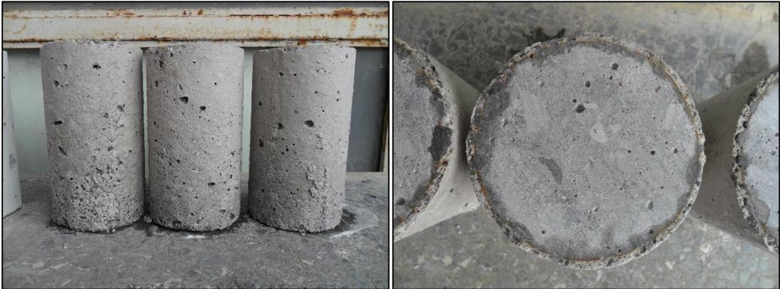
Figure 4.25. Surface deterioration of HSLWC specimens stored in sulphuric acid solution
