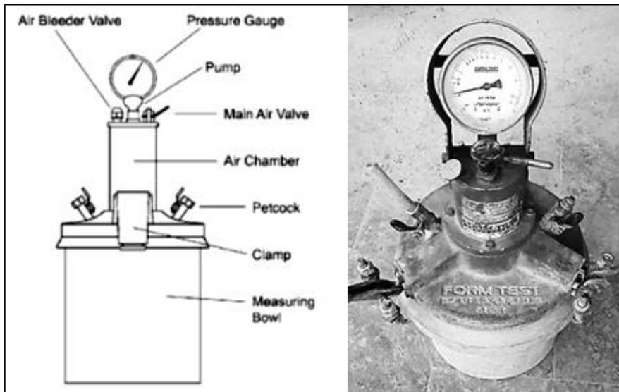
Figure 3.7. Type B air-meter with vertical air chamber (ASTM C231)
