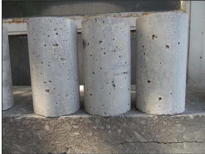
Figure 4.15. Surface deterioration of HSNWC specimens stored in magnesium sulfate solution
