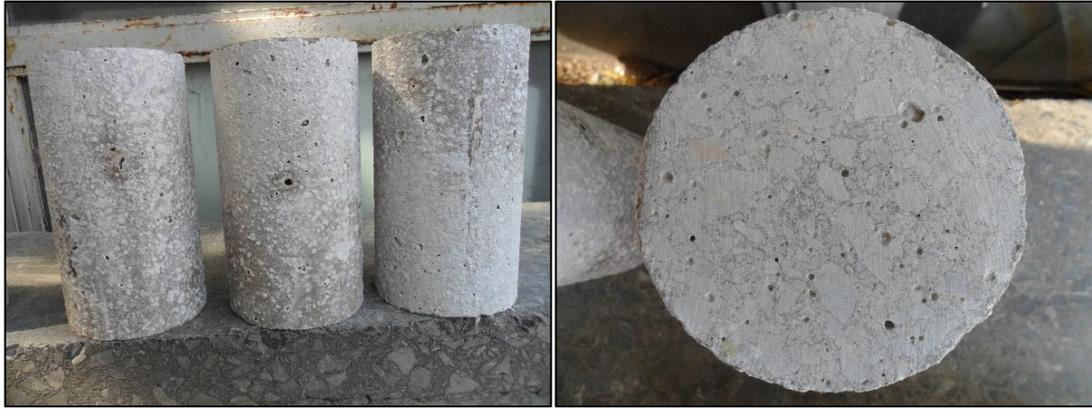
Figure 4.27. Surface deterioration of HSNWC specimens stored in sulphuric acid solution
