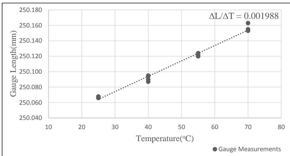
Figure 4.6. Change in gauge length with temperature change (SCLWC)
