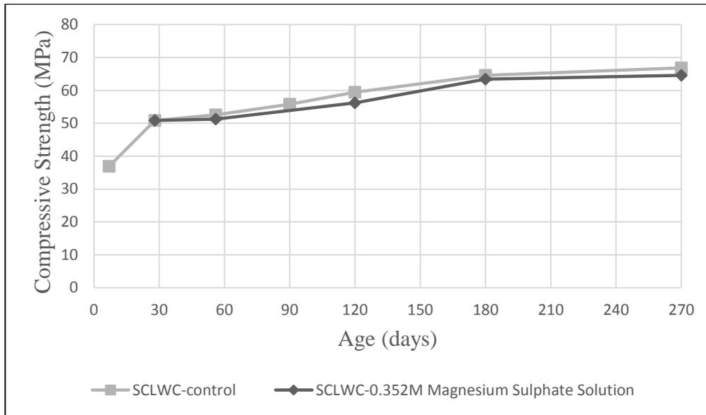
Figure 4.11. Change in compressive strength of SCLWC specimens stored in magnesium sulfate solution
