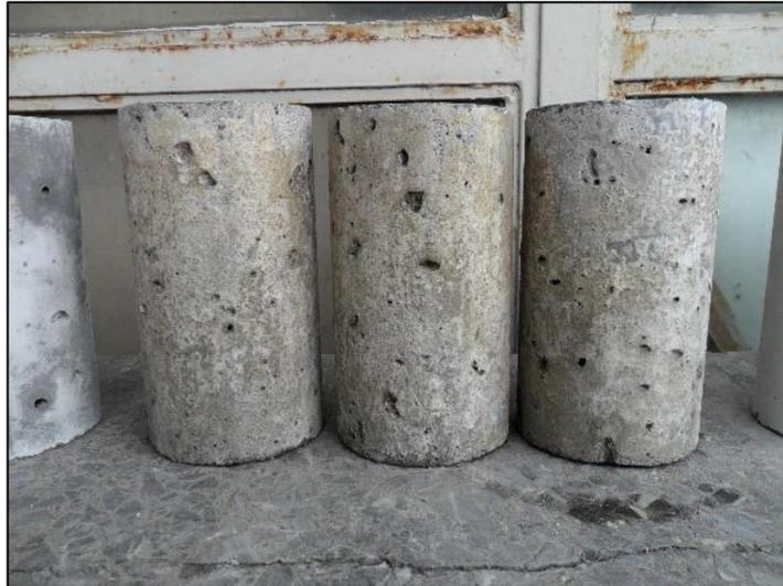
Figure 4.13. Surface deterioration of HSLWC specimens stored in magnesium sulfate solution
