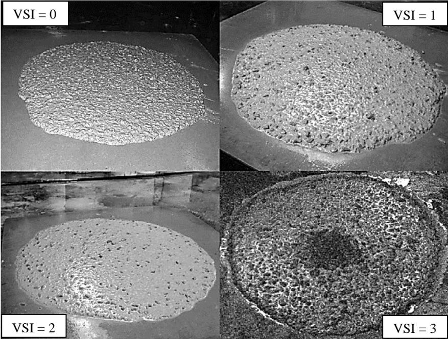
Figure 3.6. Illustration of visual stability index (ASTM C1611)
