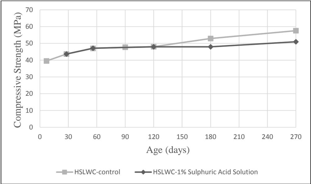
Figure 4.22. Change in compressive strength of HSLWC specimens stored in sulphuric acid solution
