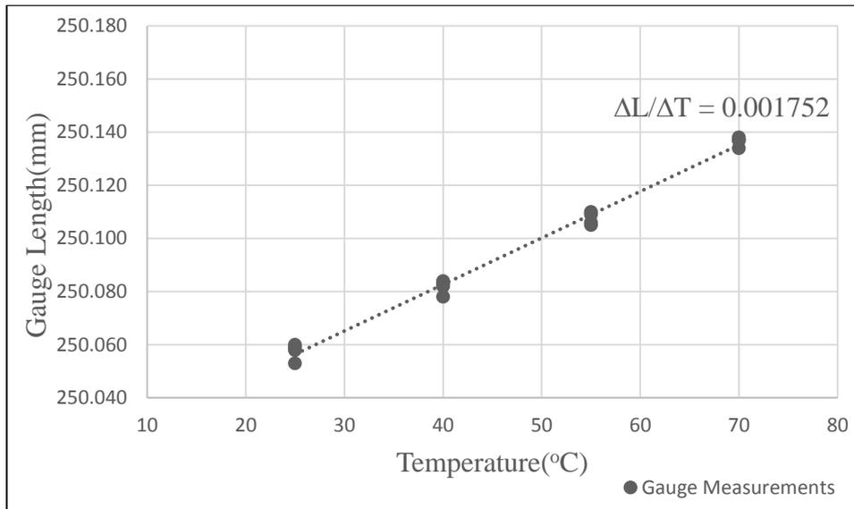
Figure 4.7. Change in gauge length with temperature change (HSNWC)
