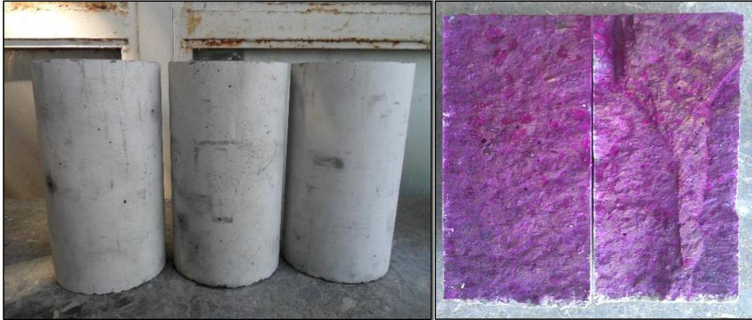
Figure 4.20. Surface deterioration of SCLWC specimens stored in sodium bicarbonate solution and interior of concrete tested by phenolphthalein
