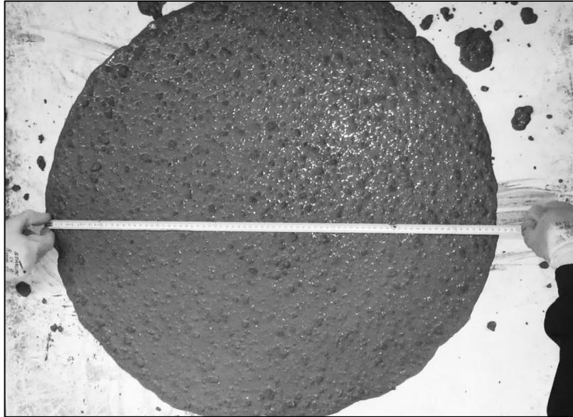
Figure 4.1. Slump flow measurement on SCLWC
