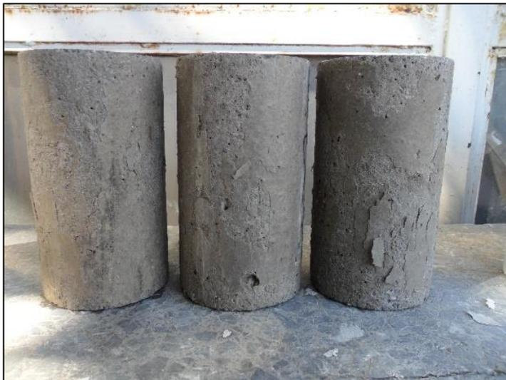
Figure 4.14. Surface deterioration of SCLWC specimens stored in magnesium sulfate solution
