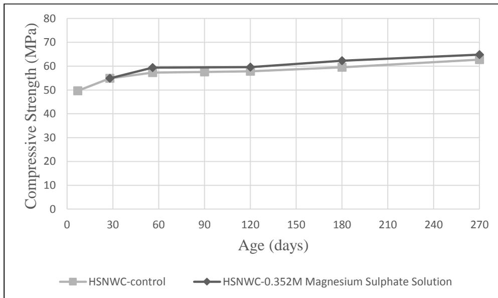
Figure 4.12 Change in compressive strength of HSNWC specimens stored in magnesium sulfate solution
