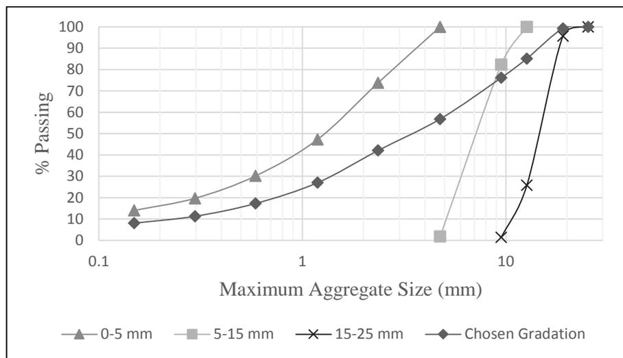
Figure 3.4. Gradation curve of limestone aggregate
