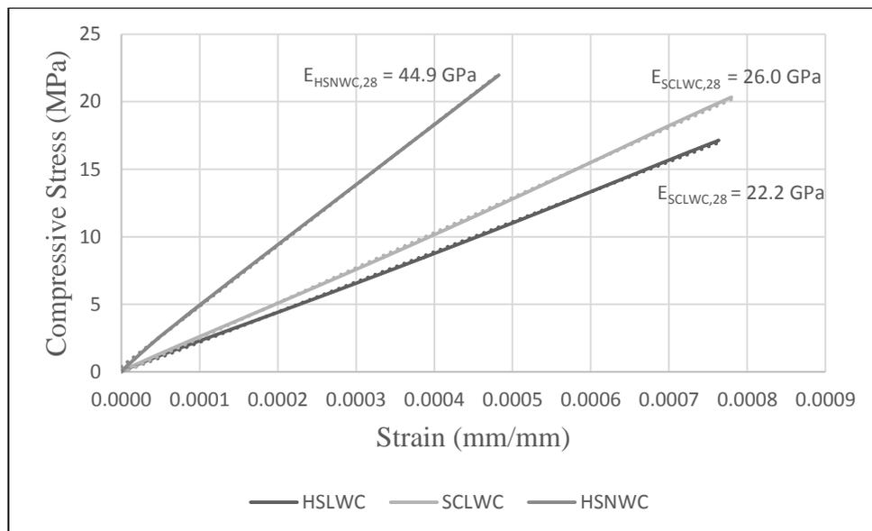
Figure 4.3. Stress-strain curves up to 40% of ultimate stress (28 days)
