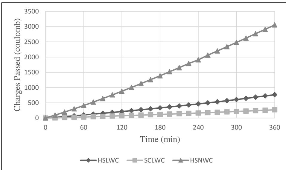
Figure 4.9. RCPT, total charges passed vs. time (90 days)
