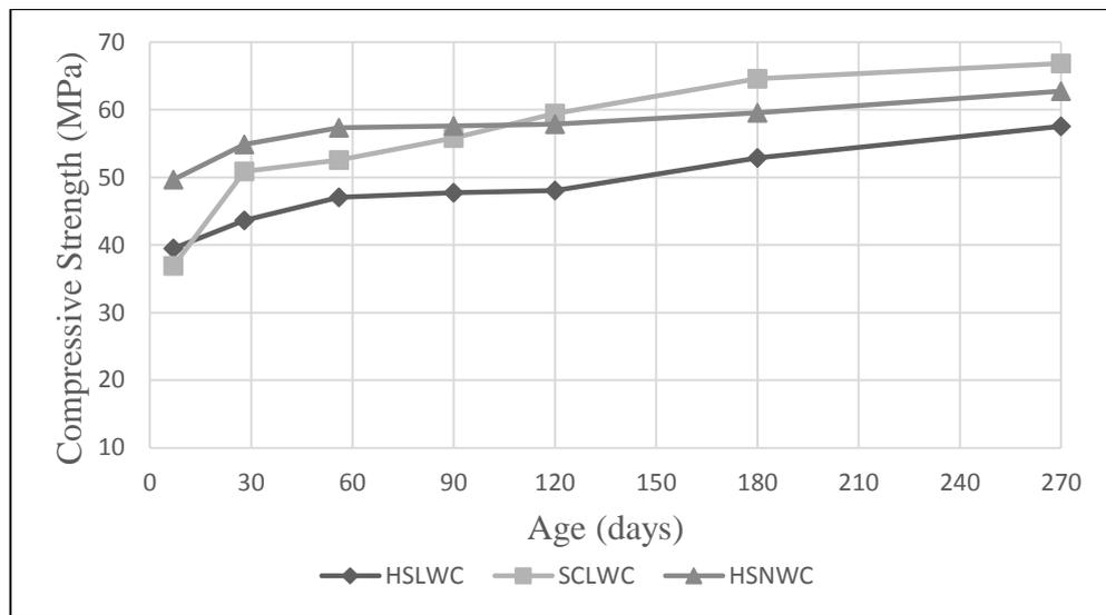
Figure 4.2. The development of compressive strength in the concrete specimens
