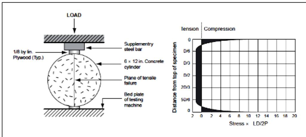
Figure 3.9. Splitting tension test and stress distribution diagram (Mehta & Monteiro, 2006)
