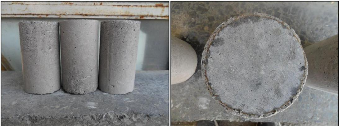
Figure 4.26. Surface deterioration of SCLWC specimens stored in sulphuric acid solution
