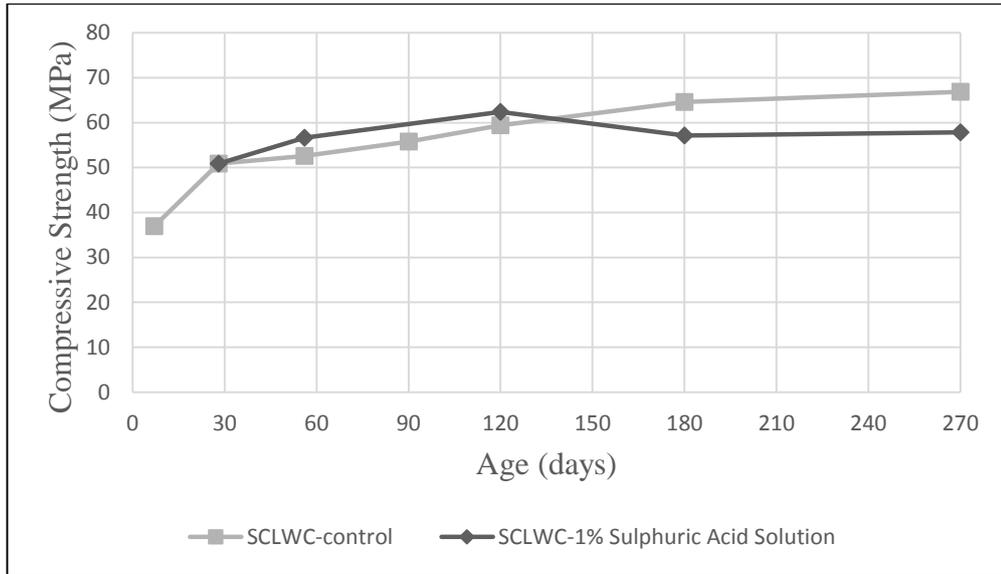
Figure 4.23. Change in compressive strength of SCLWC specimens stored in sulphuric acid solution
