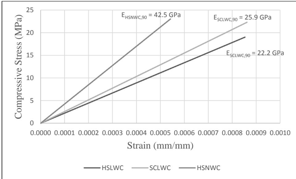
Figure 4.4. Stress-strain curves up to 40% of ultimate stress (90 days)
