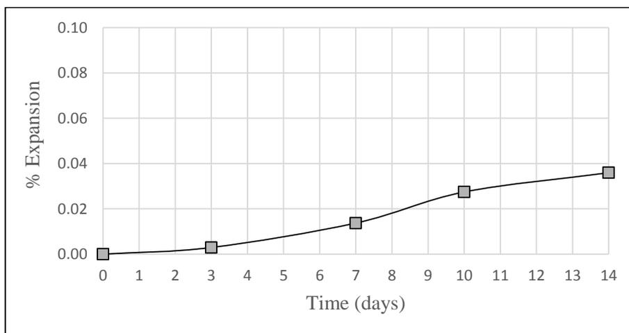
Figure 3.3. ASR expansion of perlite aggregate as determined by ASTM C1260.
