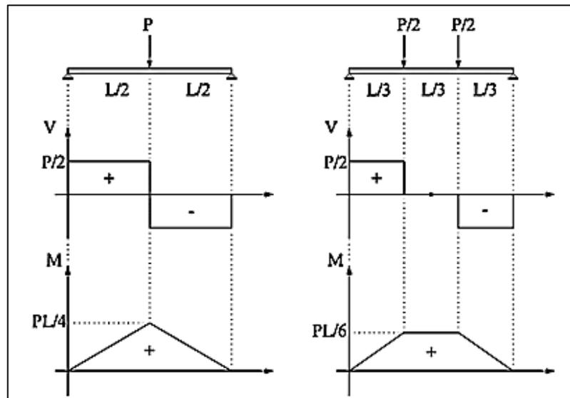
Figure 3.10. Shear and moment diagrams of CPL and TPL
