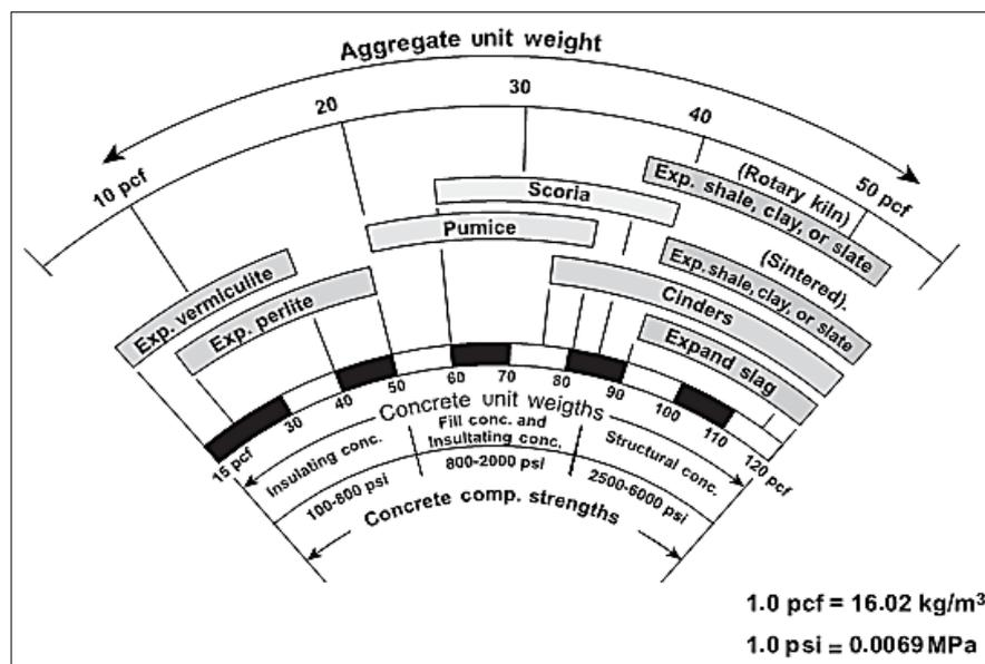
Figure 2.3. Lightweight aggregate spectrum (Mehta & Monteiro, 2006)
