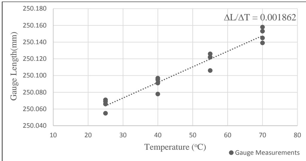
Figure 4.5. Change in gauge length with temperature change (HSLWC)
