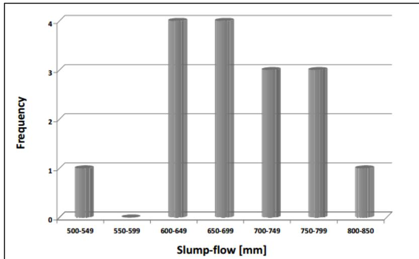
Figure 2.9. Frequency bar chart for slump-flow of self-compacting lightweight mixtures (Papanicolaou & Kaffetzakis, 2011)
