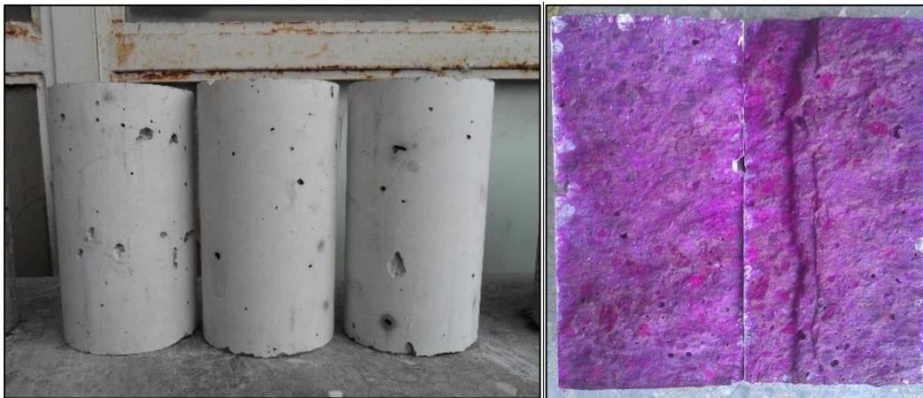
Figure 4.19. Surface deterioration of HSLWC specimens stored in sodium bicarbonate solution and interior of concrete tested by phenolphthalein
