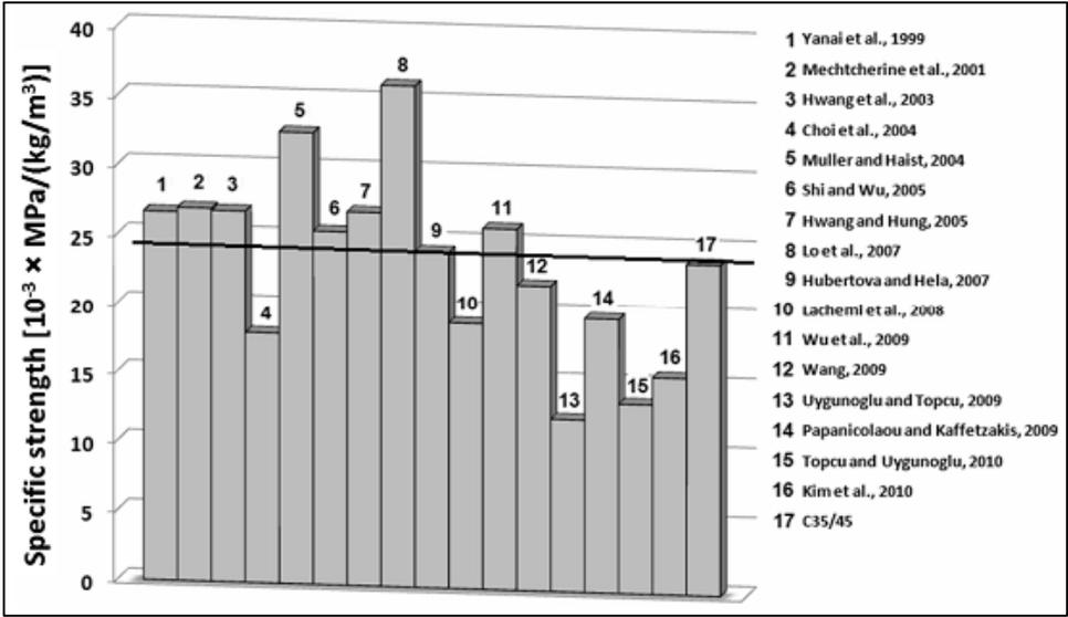
Figure 2.11. Frequency bar chart for specific strength of self-compacting lightweight mixtures (Papanicolaou & Kaffetzakis, 2011)
