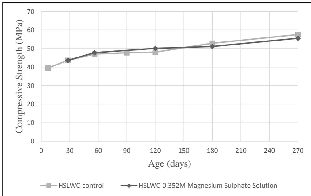
Figure 4.10. Change in compressive strength of HSLWC specimens stored in magnesium sulfate solution
