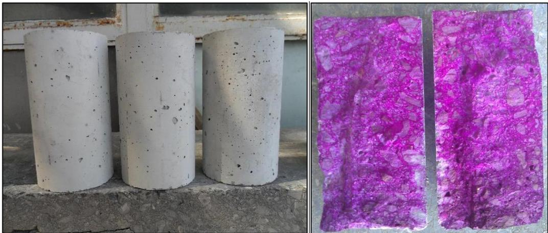
Figure 4.21. Surface deterioration of HSNWC specimens stored in sodium bicarbonate solution and interior of concrete tested by phenolphthalein
