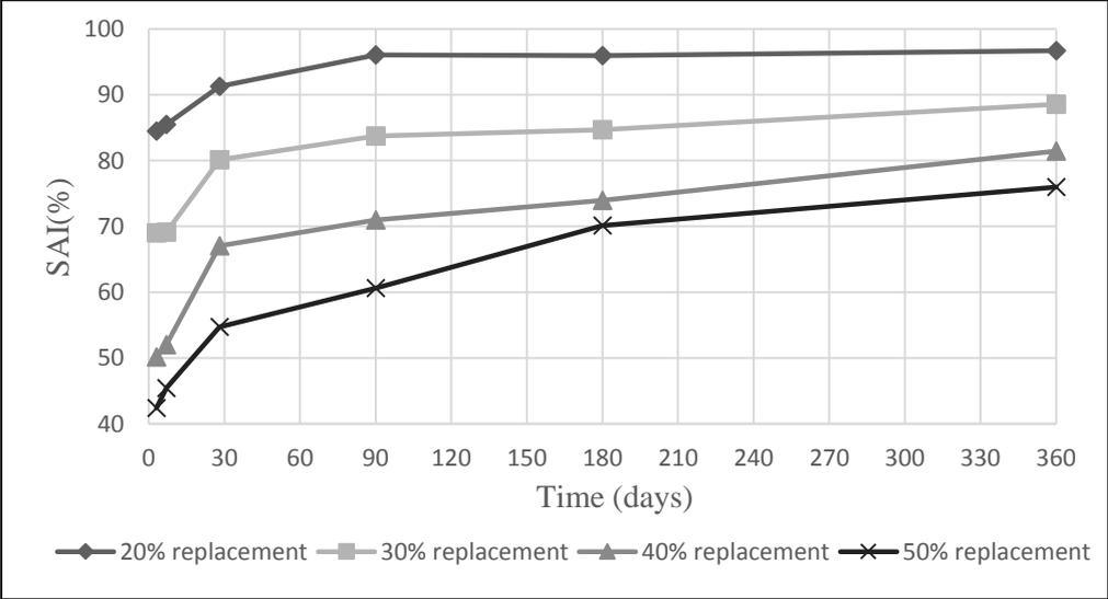
Figure 3.1. Strength activity index of perlite powder versus time
