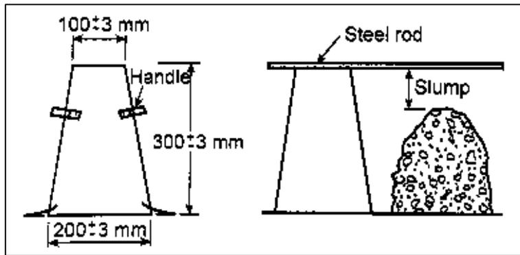
Figure 3.5. Slump cone and measurement of slump (Erdoğan, 2005)
