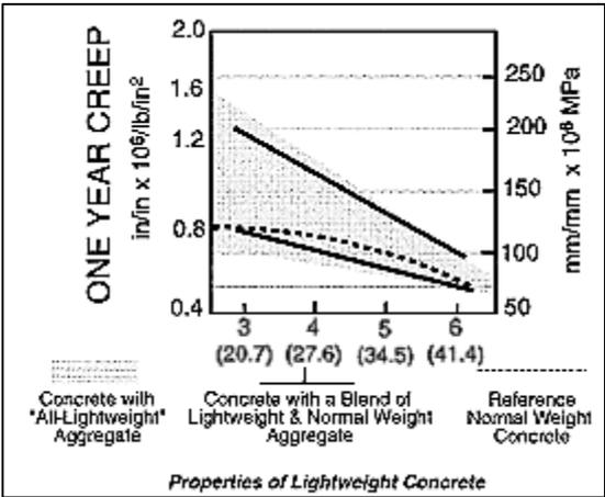
Figure 2.5. Creep of moist-cured lightweight concrete with respect to compressive strength (ACI Committee 213, 2003)
