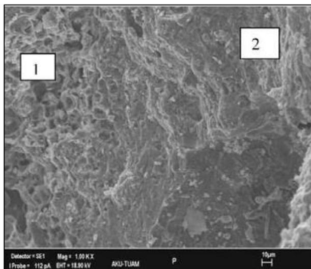
Figure 2.8. Microstructure of self-compacting concrete with natural pumice aggregate (1: aggregate, 2: cement paste matrix) (Topçu & Uygunoğlu, 2010)
