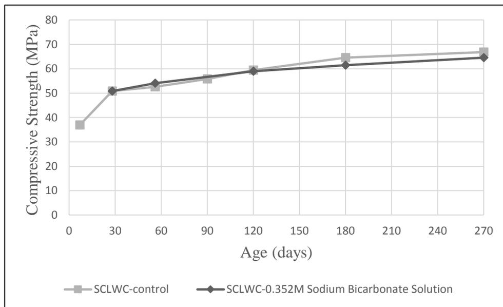
Figure 4.17. Change in compressive strength of SCLWC specimens stored in sodium bicarbonate solution
