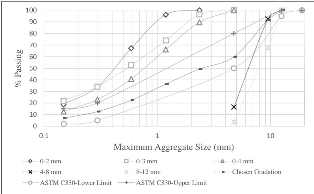
Figure 3.2. Gradation curve of perlite aggregate
