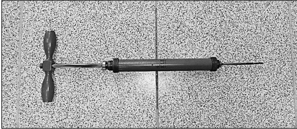
Figure 3.8. Concrete setting time testing apparatus
