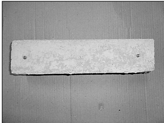
Figure 3.11. Beam specimen for thermal expansion experiment
