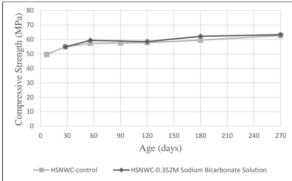
Figure 4.18. Change in compressive strength of HSNWC specimens stored in sodium bicarbonate solution
