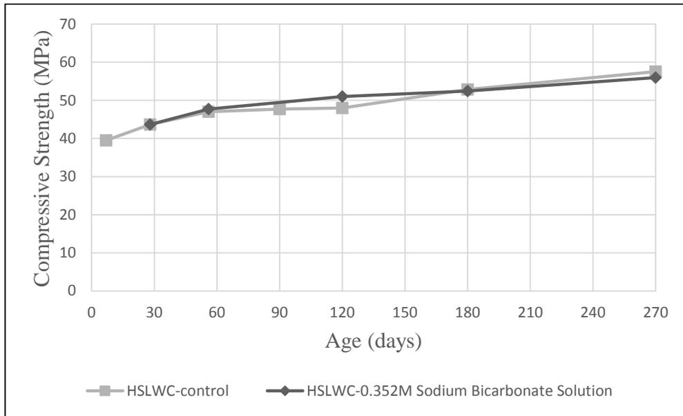
Figure 4.16. Change in compressive strength of HSLWC specimens stored in sodium bicarbonate solution
