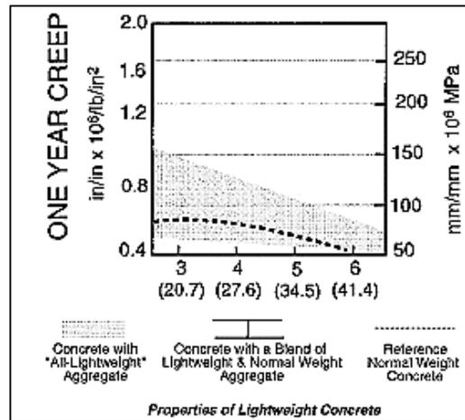
Figure 2.6. Creep of steam-cured lightweight concrete with respect to compressive strength (ACI Committee 213, 2003)
