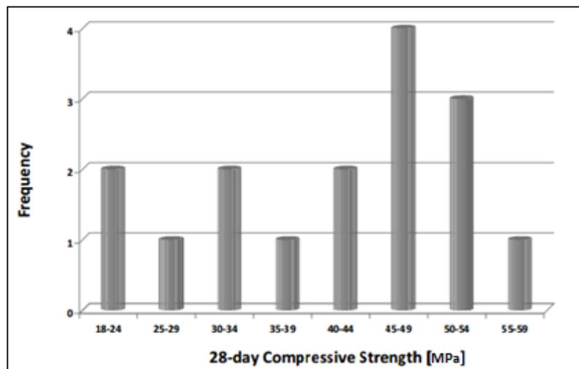
Figure 2.10. Frequency bar chart for 28-day compressive strength of self-compacting lightweight mixtures (Papanicolaou & Kaffetzakis, 2011)
