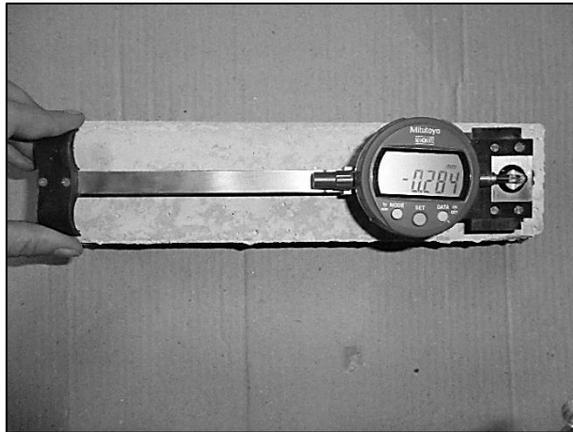
Figure 3.12. Measurement of thermal expansion of concrete specimens
