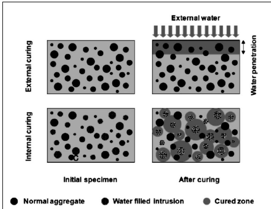
Figure 2.4. The movement of moisture in external and internal curing (Castro, De la Varga, Golias, & Weiss, 2010)
