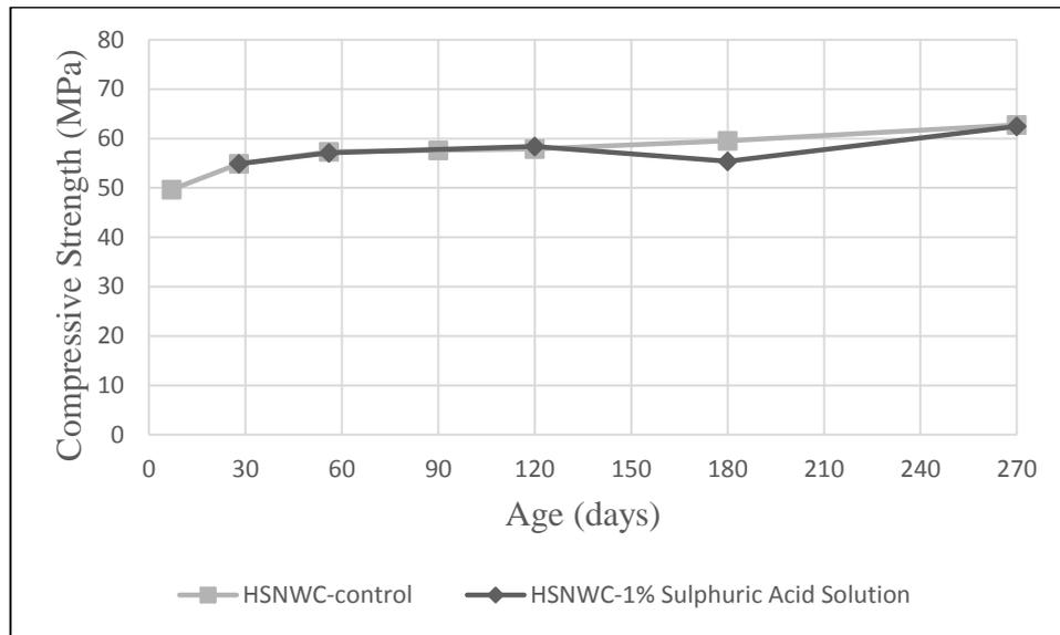
Figure 4.24. Change in compressive strength of HSNWC specimens stored in sulphuric acid solution
