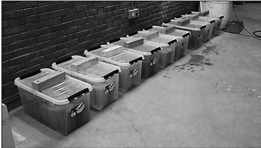
Figure 3.13. Storage of concrete specimens in aggressive chemical solutions
