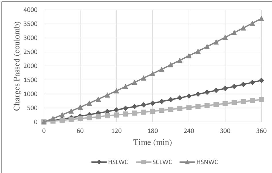
Figure 4.8. RCPT, total charges passed vs. time (28 days)
