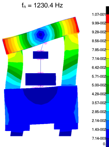
Figure 3.16 Comparison of the tenth mode of finite element model and fourth mode of analytical model for the design configuration given in Table 3.4
