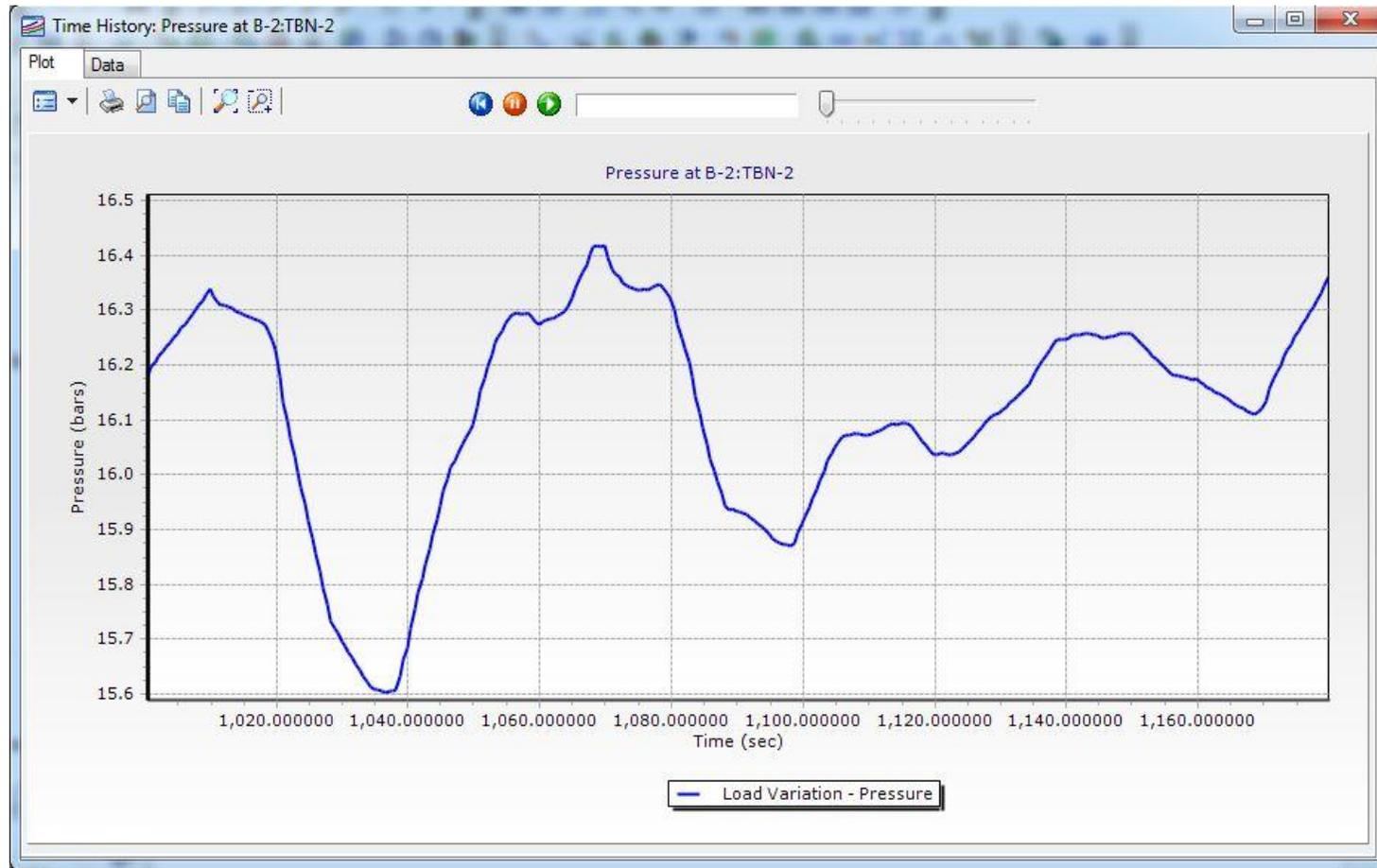
Figure 4.7 Transient Time History of Pressure at Turbine
