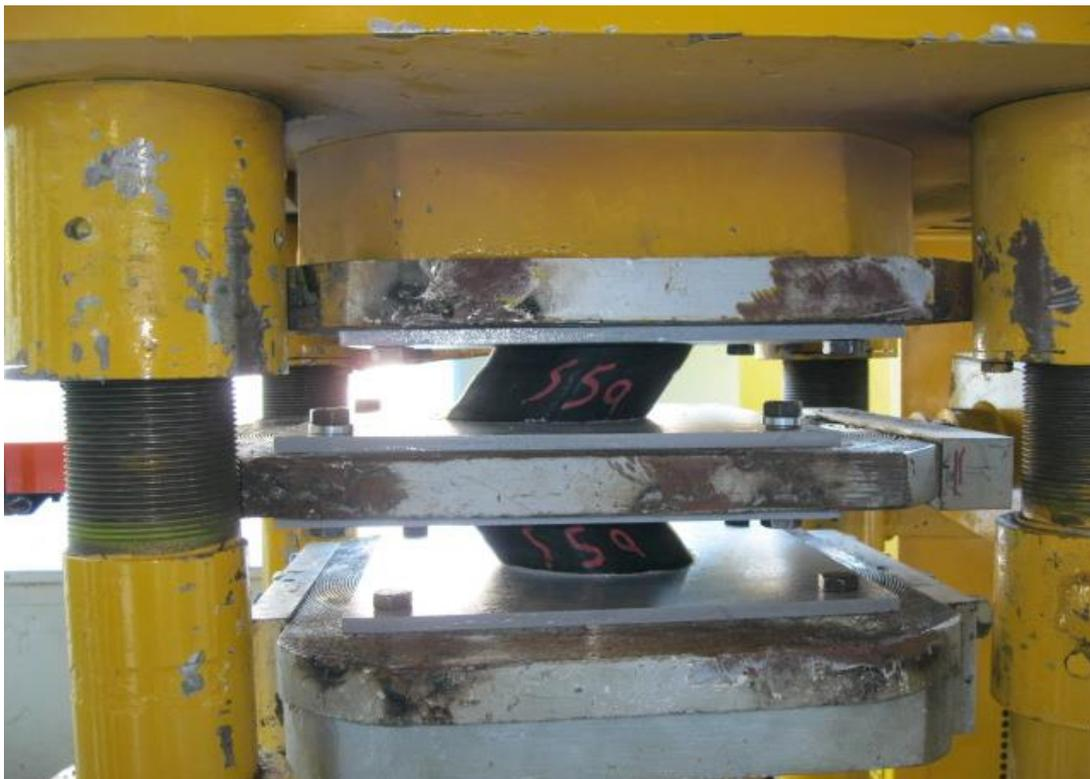
**Figure 4.9** B-St-C150-1 under vertical pressure and 100% shear strain
