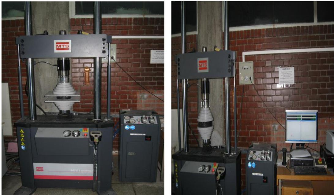
**Figure 3.5** Vertical compression test setup
