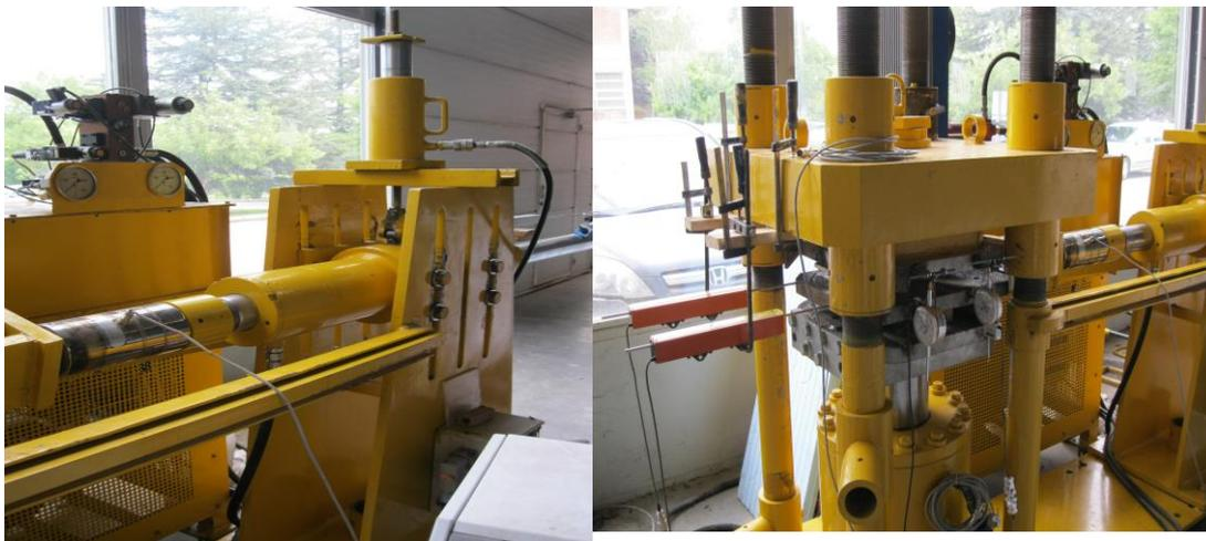
**Figure 3.3** Loading and measuring systems
