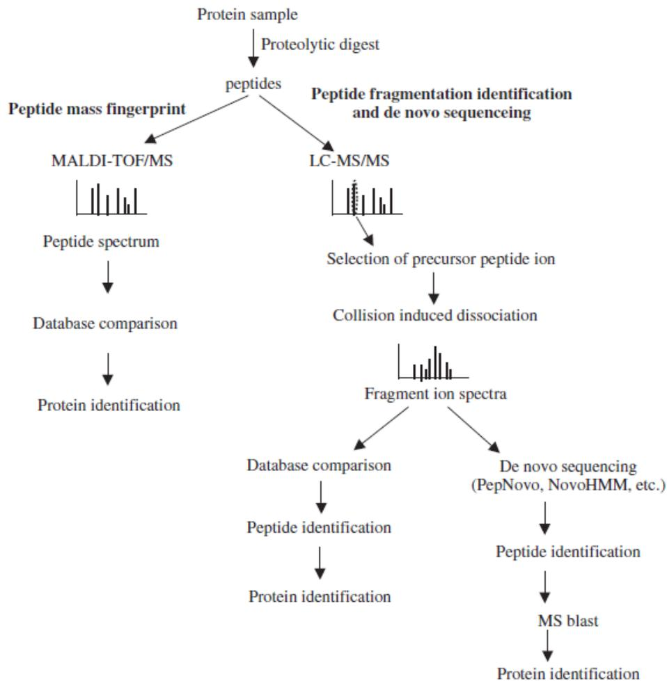
**Figure 1.10** Differences between PMF, peptide fragmentation identification, and de novo sequencing (Agrawal & Randeep, 2008)
