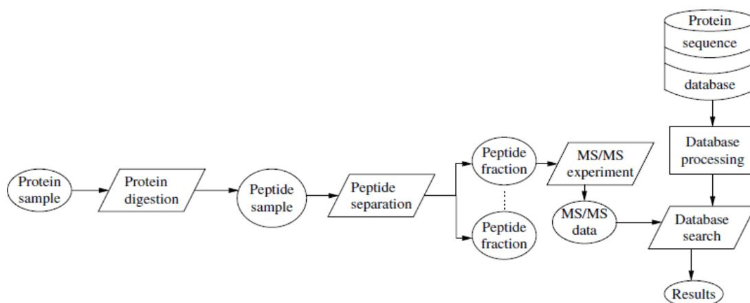
**Figure 1.8** MS/MS protein analysis approach (for peptide residues) (Eidhammer et al, 2007).
