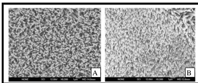
**Figure 1.3** SEM images of ZnO nanorods grown on glass substrates coated with gold (A) The ZnO nanorods only and (B) ZnO nanorods with immobilized GAO enzyme (Khun *et al.*, 2012).
