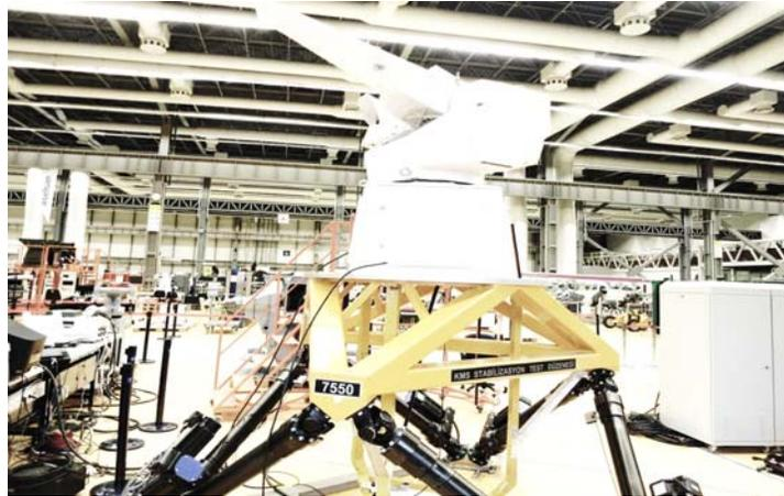
Figure 5.2 The Gyro stabilized platform mounted on a Stewart platform (Photo Courtesy of ASELSAN Inc.)
