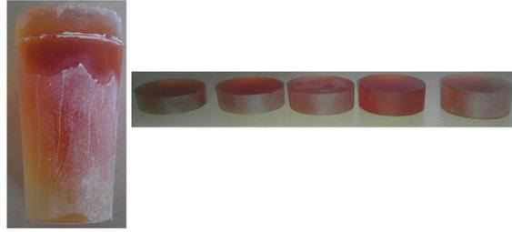
Figure 4.3 The main coupling material and the other samples cutted with lathe at different thicknesses (Test 1)
