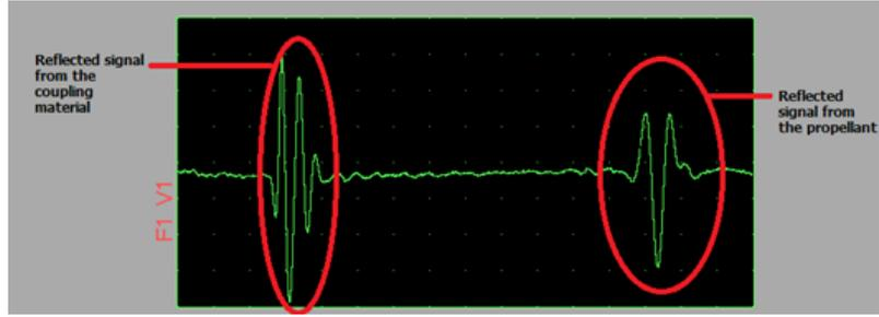
Figure 7.13 Reflected signals for Test 4 at the initial time
