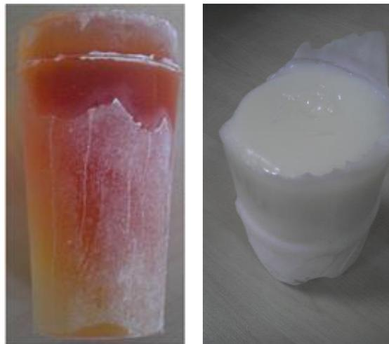
Figure 5.4 Coupling material; for propellants with aluminum (right), for propellants without aluminum (left)
