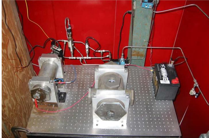
Figure 3.1 Crawford bomb mechanism with strand burner [32]
