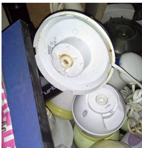
Figure 30 - Broken choppers with eroded gears.
