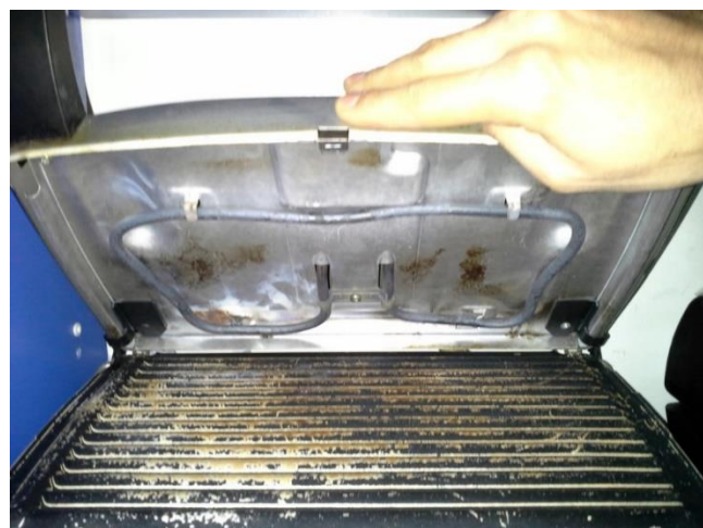
Figure 32 - Sandwich toaster with eroded teflon layers.
