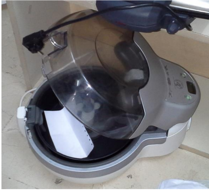
Figure 38 - Cleaning of deep fryers is difficult as a result of this oil leaks into the motor.
