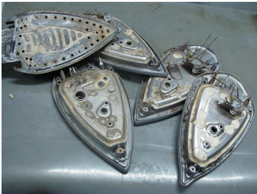
Figure 21 - Iron base is broken-down as a result of calcification.
