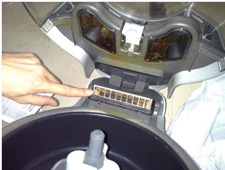
Figure 39 - Filter of the deep fryer that is covered with oil and dirt.
