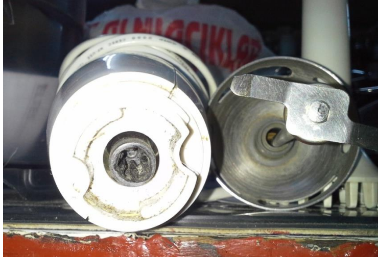
Figure 26 - Blender with eroded shaft gear.
