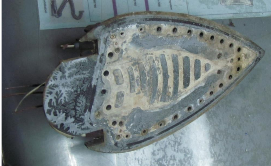
Figure 20 - Iron base is broken-down as a result of calcification.
