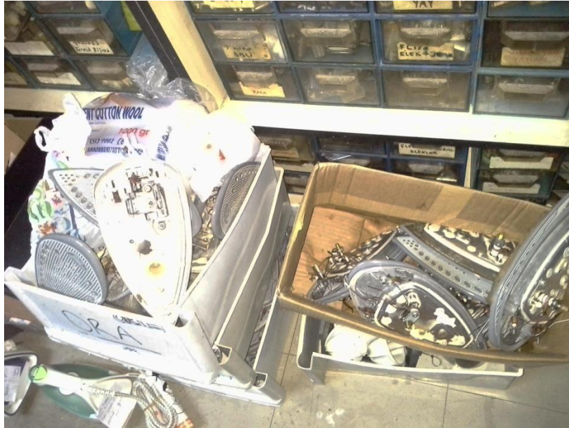
Figure 22 - Disassembled bases from broken irons.
