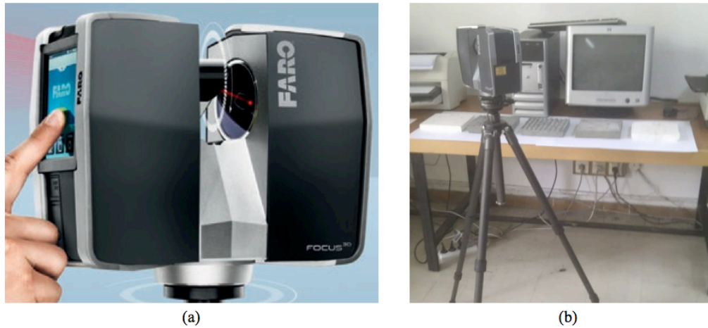
Figure 3.11. (a) Faro Focus 3-D laser scanner. (b) 3-D laser scanner setup.
