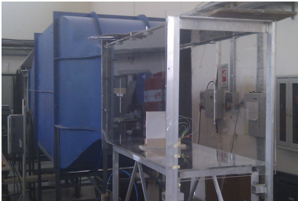
Figure 3.8. Test chamber that is attached to the wind tunnel with a rotating sample holder.
