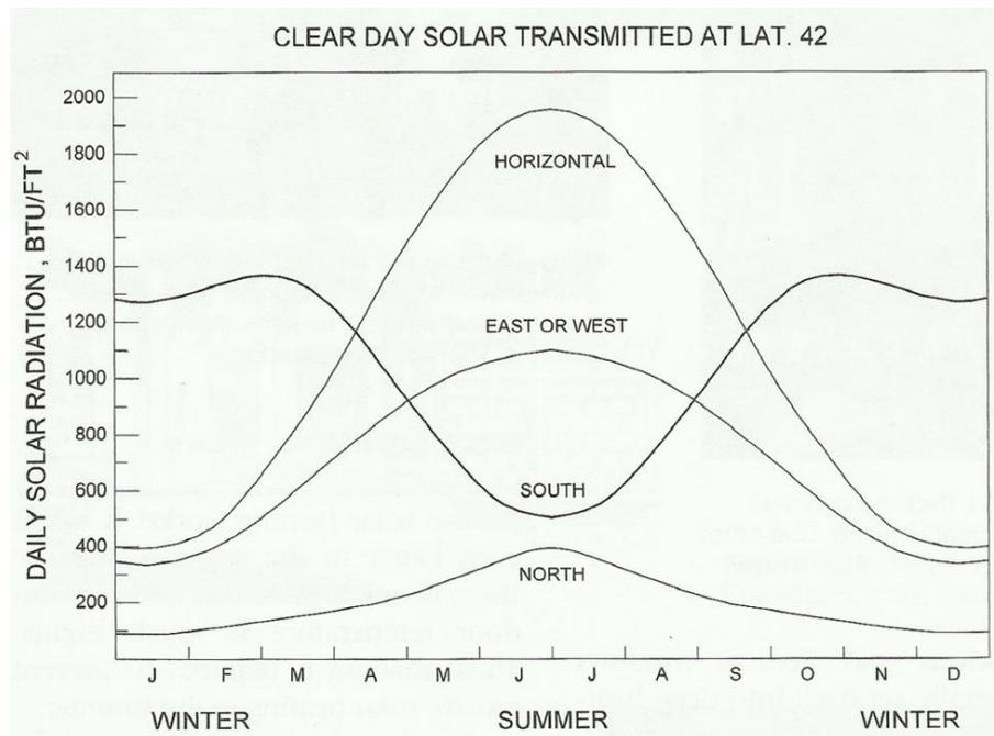
**Figure 2.15** Solar Radiation According to Orientation (Lechner, 2001)
