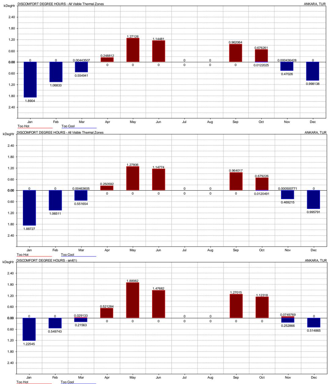
**Figure B.1** DDH for the Classroom with WS1 (Top), WS2 (Middle) and WS3 (Bottom)
