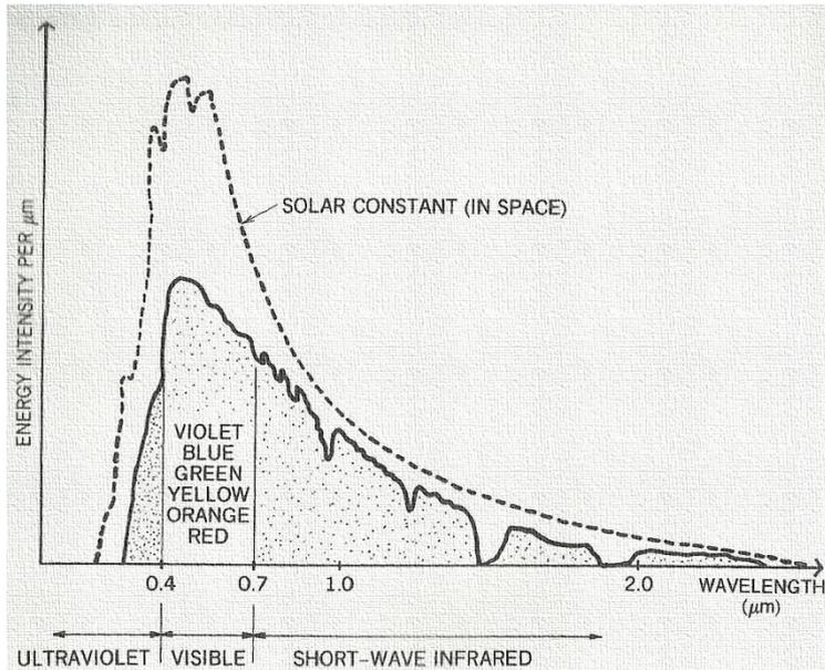
**Figure 2.1** The Solar Spectrum (Lechner, 2001)
