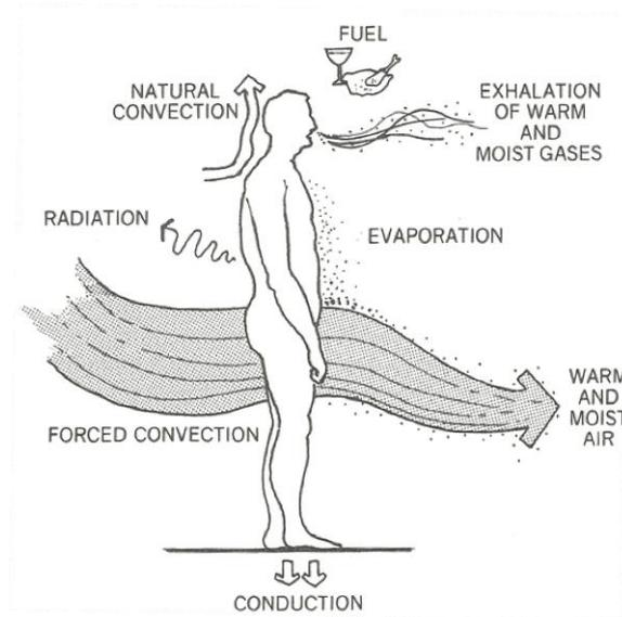
**Figure 2.12** Heat Exchange Method of a Body (Lechner, 2001)
