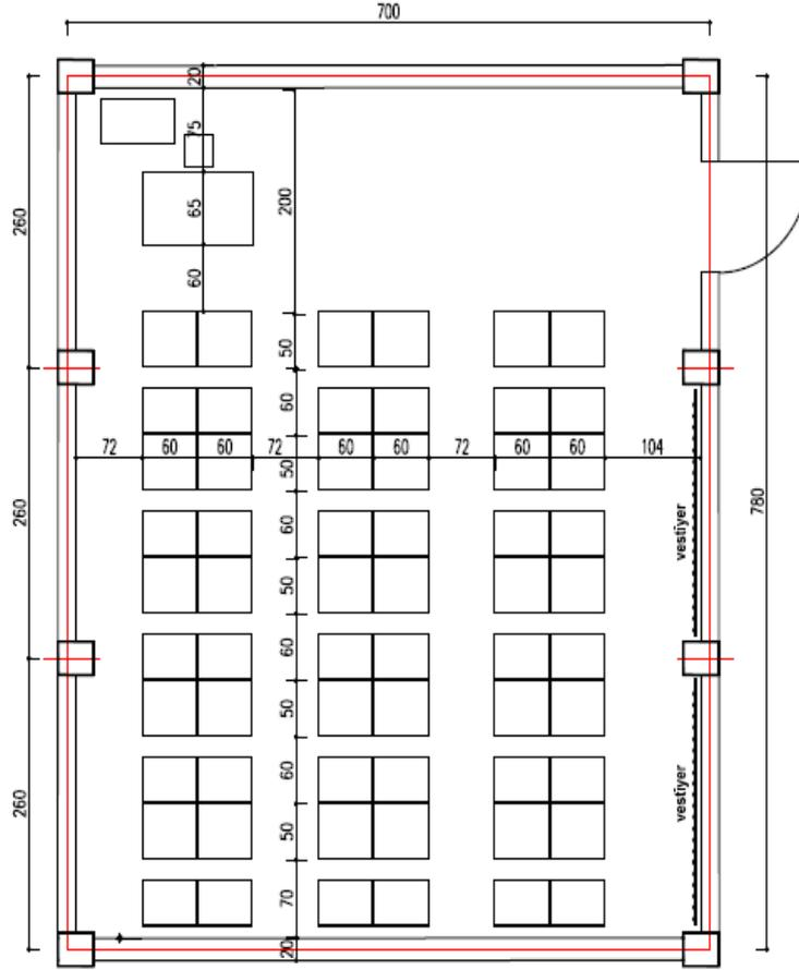
**Figure 3.1** Architectural Drawing of a Typical Classroom
