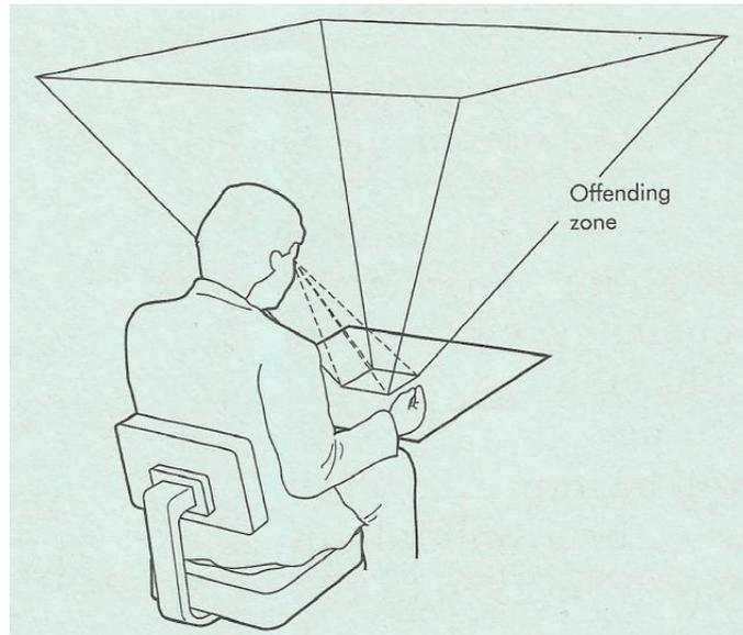
**Figure 2.11** Schematic Diagram of Offending Zone (CIBSE, 1994)
