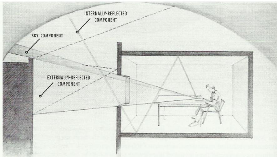
**Figure 2.6** Three Components Comprising Daylight Factor (Heerwagen, 2004)
