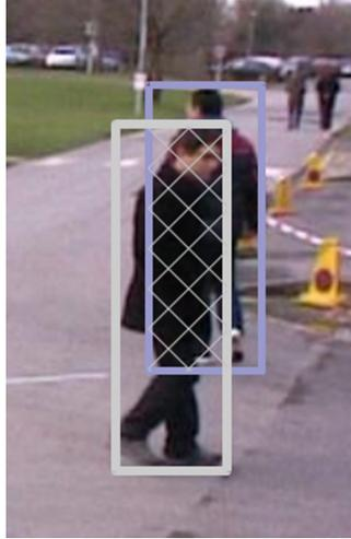
Figure 3.4: Illustration of the occlusion probability estimation. The person with gray bounding box is occluding the one with light blue bounding box. The occlusion probability of the person closer to the camera is taken as zero, while that of the farther is computed as the ratio of the hatched area to the area of the light blue bounding box.
