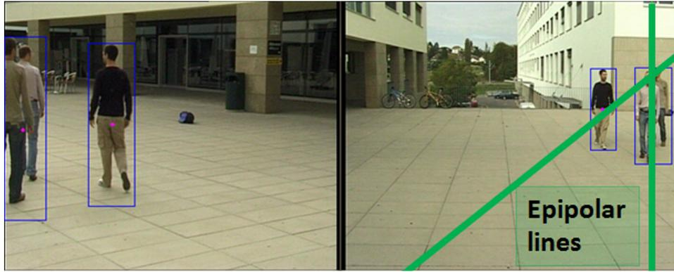
Figure 3.3: Illustration of the epipolar mismatch cost. There are two silhouettes to consider on each view, which makes four pairs. The epipolar lines with respect to the centroids on the left view are drawn on the right view. The distances of the two centroids to these two lines, both on the right view, constitute the epipolar mismatch costs for the four pairs for the right view.
