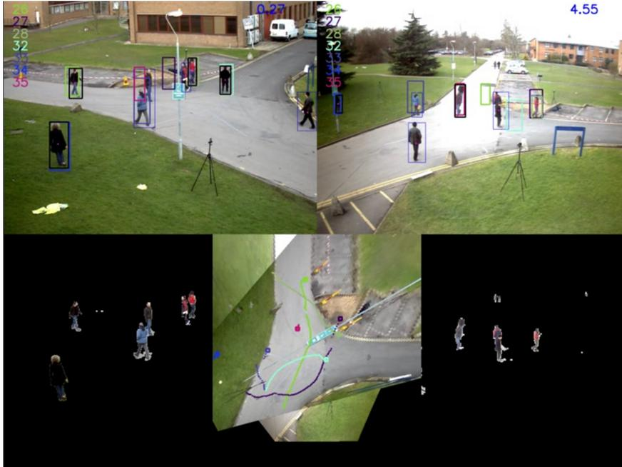
Figure 4.5: Illustration of the tracking error made when tracking a maneuvering object. The tracking is performed as described in this chapter. The frame difference is equal to 5 frames. The man dressed in black at the junction loses his track shown in light blue, since he started moving back in the right view and remains stationary in the left. Time difference compensation cannot work effectively with maneuvering objects, especially when time difference is large.
