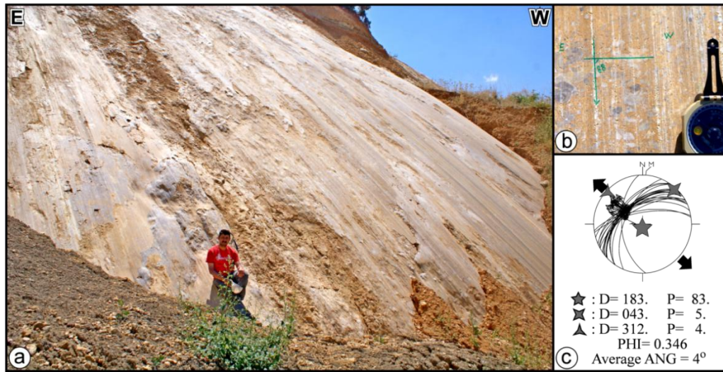
Figure 4.25. Field view of the eastern tip of the Yaka Fault Zone (YAFZ) (a). Well-developed slickenline on the fault surface (b) and stereographic plot of these slip data on the Schmidt's lower hemisphere net (c).
