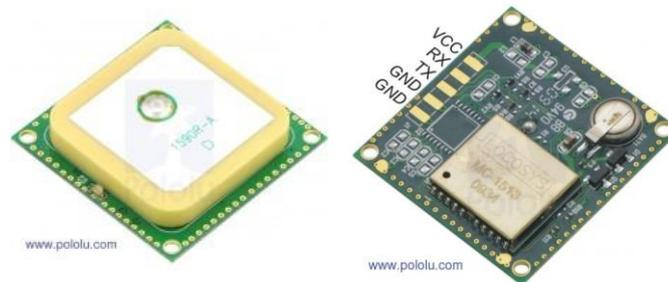
Figure 57 - 66-Channel LS20031 GPS Receiver Module [54]
