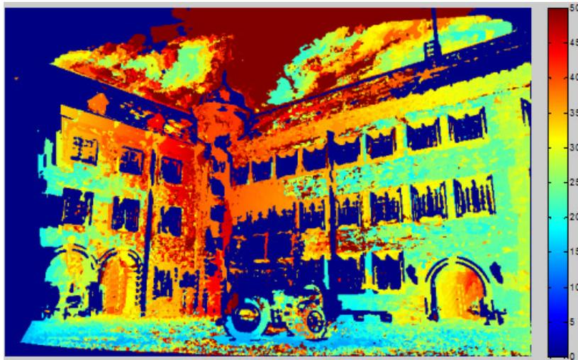
Figure 3.10: Colored depth representation as result of plane sweeping with depth sampling for the images in Figure 3.6.
