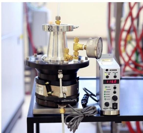
**Figure 3.4** Photograph of the vibrational powder feeder system.
