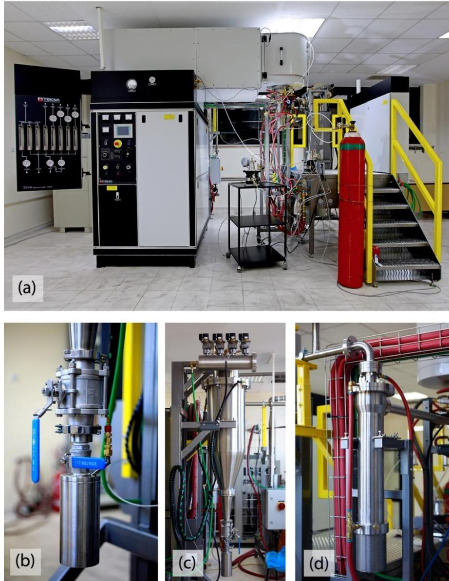
**Figure 3.7** Photographs of (a) induction plasma system, (b) detachable and airtight powder collector, (c) powder collection unit and (d) cyclone unit.
