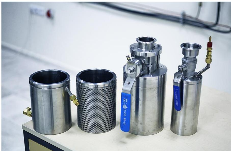
**Figure 3.8** Photograph showing the bottom collector, cyclone collector, large and small capacity powder collector, respectively (from left to right).
