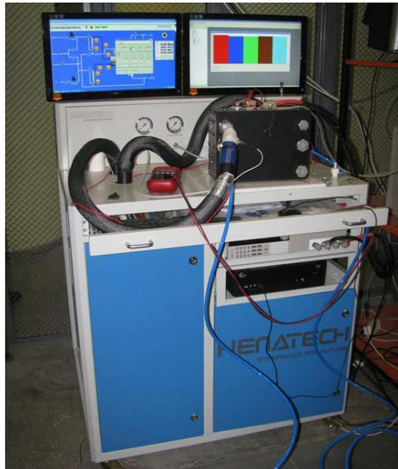
Figure 5.19 HENATECH Test Station connected to short stack (5 cells)
