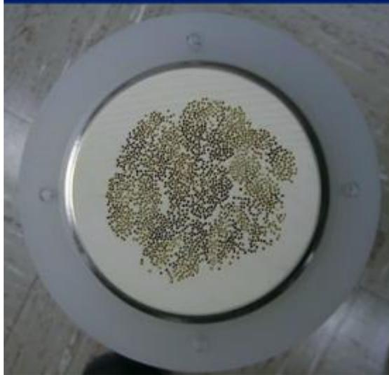
Figure 3.4 Cross section of the Nafion tubes in the humidifier
