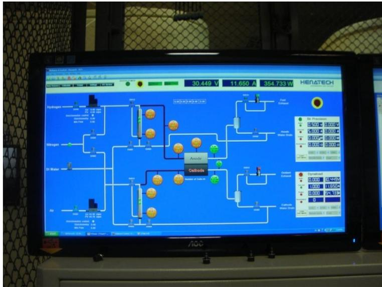
Figure 5.24 A typical screen shot during performance test of 3kW PEMFC stack.
