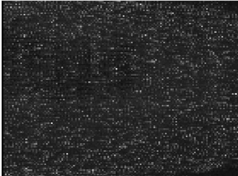
Figure 3.13: Average image noise over the array for the third design revision of the 160x120 low-cost sensor. The noise is averaged over 64 frames.
