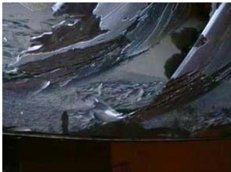
Figure 2.2 Damaged Francis runners caused by silt and sand (Gummer, 2009)
