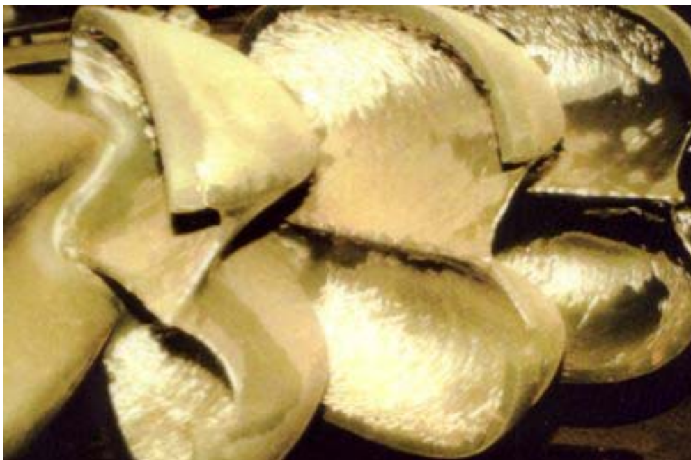
Figure 2.1 Damaged Pelton buckets caused by silt and sand (Ardüser and Karcheter, 2009)
