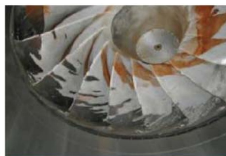
Figure 2.3 Abrasion damage to the turbine runners (Khatsuria, 2012)
