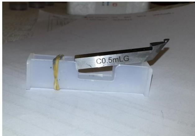
Figure 3.5 Tool numbering for monocrystalline diamond tool
