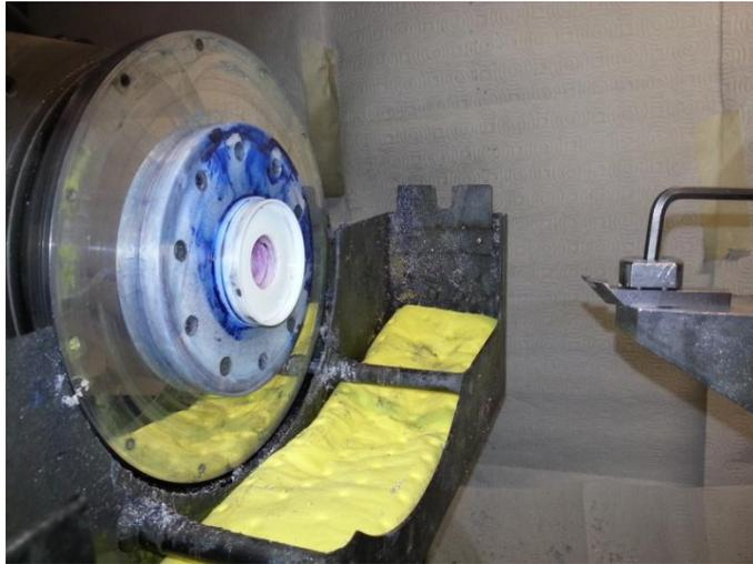
Figure 3.4 Mounting of monocrystalline diamond tool
