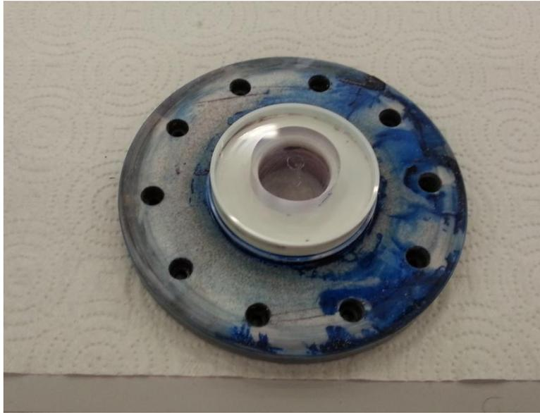
Figure 3.10 Fixture for the placement of PC specimen
