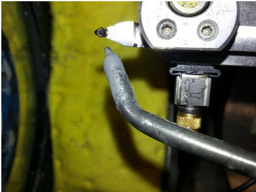
Figure 3.7 Mounting of the accelerometer (Top view)
