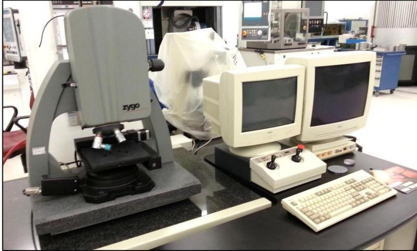
Figure 3.15 Zygo NewView 5000 White Light Interferometry [70]
