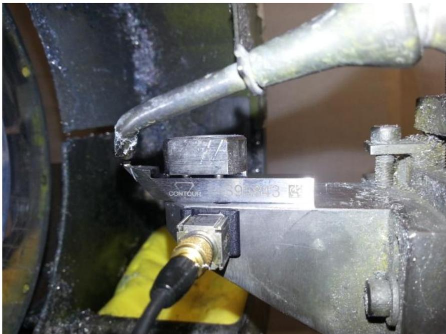
Figure 3.8 Mounting of the accelerometer (Front view)
