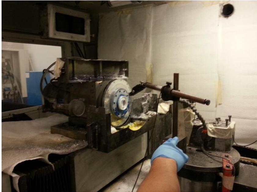
Figure 3.11 Centering of the PC specimen
