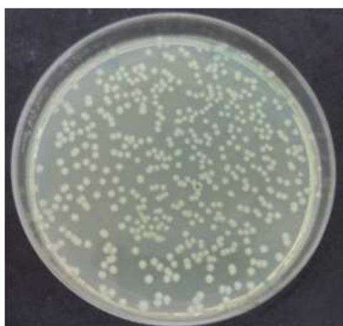
Figure 4.12 Number of E.coli cells survived on the uncoated textile ( 275 \pm 5 CFU/100 \mu\text{l} were counted)
