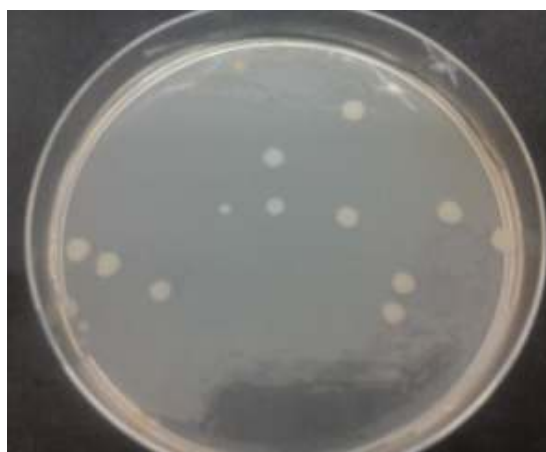
Figure 4.39 Number of B.atrophaeus cells survived on the \text{TiO}_2 coated textile (11 \pm 2 CFU/100 \mu l were counted)
