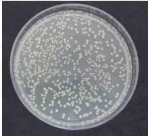
Figure 4.44 Number of B.atrophaeus cells survived on the textile that was coated and doped with tungsten and zinc ( 586 \pm 4 CFU/100 \mu l were counted)
