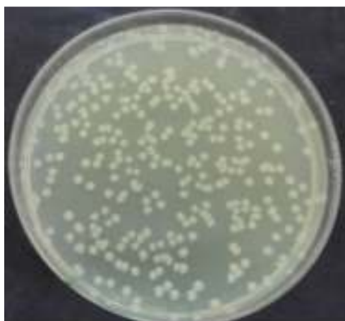
Figure 4.14 Number of E.coli cells survived on the textile that uncoated ( 298 \pm 5 CFU/100 \mu\text{l} were counted)
