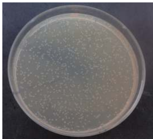
Figure 4.40 Number of S.aureus cells survived on the textile that was coated with W doped \text{TiO}_2 ( 715 \pm 4 CFU/100 \mu\text{l} were counted)
