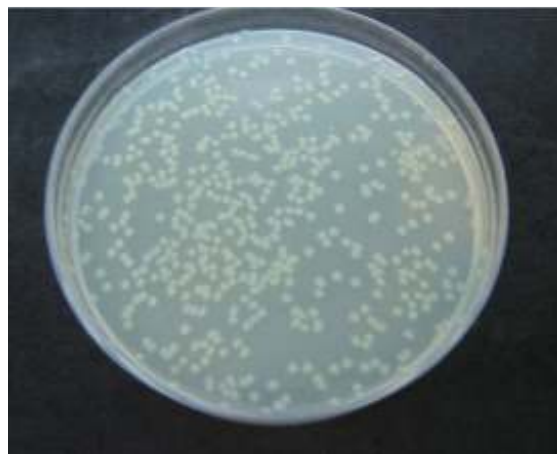
Figure 4.5 Number of E.coli cells in the microbial suspension of 1 ml applied on the uncoated surface/suspension and illuminated with 10^{-4} dilution that have 0.1 optical density value [ 240 \pm 8 CFU/100 \mu l]
