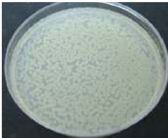
Figure 4.80 Number S.aureus of cells survived on the 200 µg/ml zeolite containing plate [ 820 \pm 7 CFU/100 µl]
