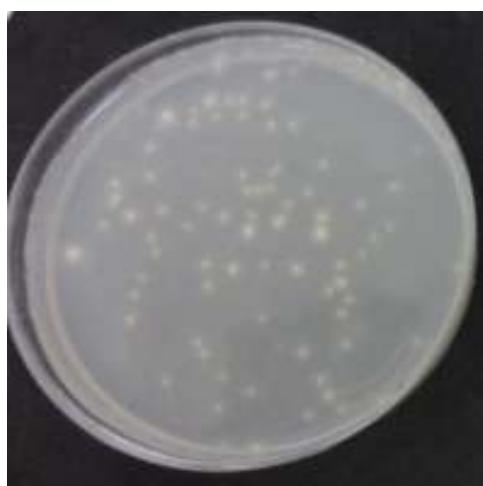
Figure 4.70 Number of A.niger cells survived on the textile that was coated and doped with tungsten and zinc ( 40 \pm 2 CFU/100 \mu l were counted)
