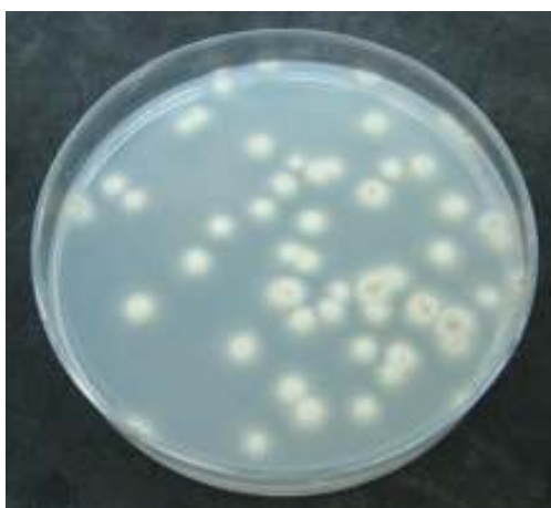
Figure 4.62 Number of A.niger cells survived in the TiO 2 powder containing suspension ( 47 \pm 3 CFU/100 \mu l were counted)
