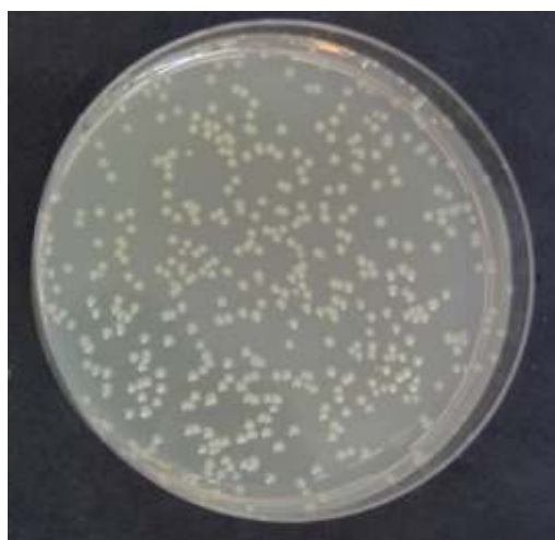
Figure 4.17 Number of E.coli cells survived on the textile that was uncoated (304 \pm 6 CFU/100 \mu l were counted)
