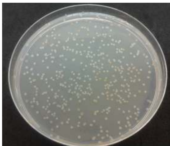
Figure 4.41 Number of B.atrophaeus cells survived on the textile that was coated with W doped \text{TiO}_2 ( 582 \pm 5 CFU/100 \mu\text{l} were counted)
