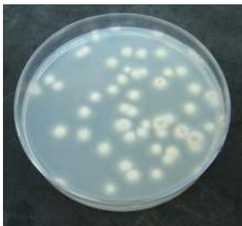
Figure 4.65 Number of A.niger cells survived on the \text{TiO}_2 coated textile ( 51 \pm 3 CFU/100 \mu l were counted)
