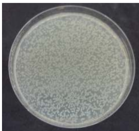
Figure 4.27 Number of S.aureus cells survived on the textile that was coated with W doped \text{TiO}_2 ( 715 \pm 3 CFU/100 \mu\text{l} were counted)
