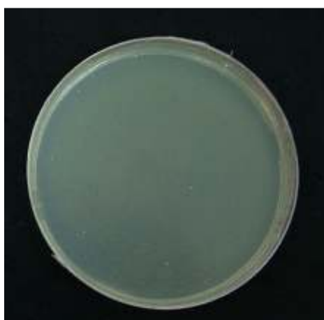
Figure 4.83 Number of B.atrophaeus spores survived on the 500 µg/ml zeolite containing plate [83±4 CFU/100 µl]
