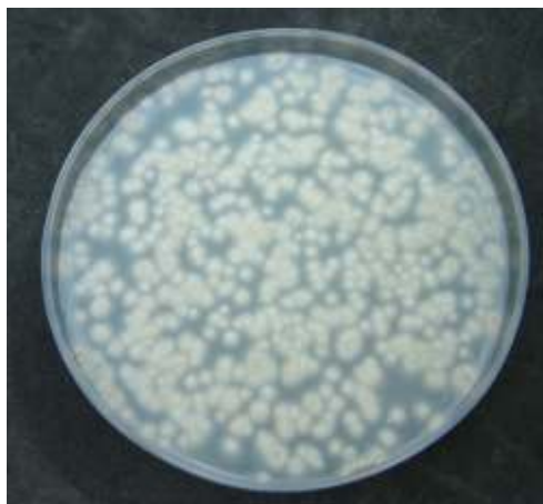
Figure 4.69 Number of A.niger cells survived on the textile that was uncoated ( 402 \pm 5 CFU/100 \mu l were counted)
