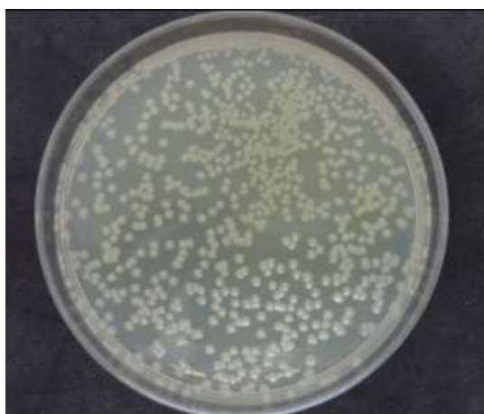
Figure 4.81 Number of S.aureus cells survived on the 200 µg/ml silver zeolite containing plate [ 266 \pm 5 CFU/100 µl]
