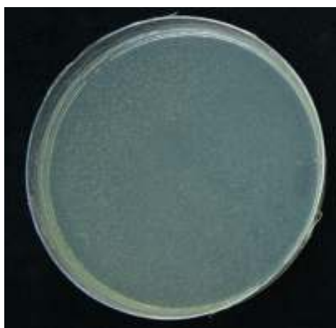
Figure 4.82 Number B.atrophaeus of spores survived on the 500 µg/ml zeolite containing plate [833±6 CFU/100 µl]
