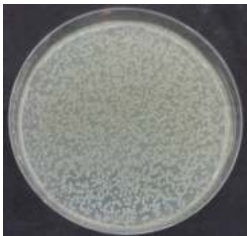
Figure 4.25 Number of S.aureus cells survived on the uncoated textile (734 ±3 CFU/100 µl were counted)
