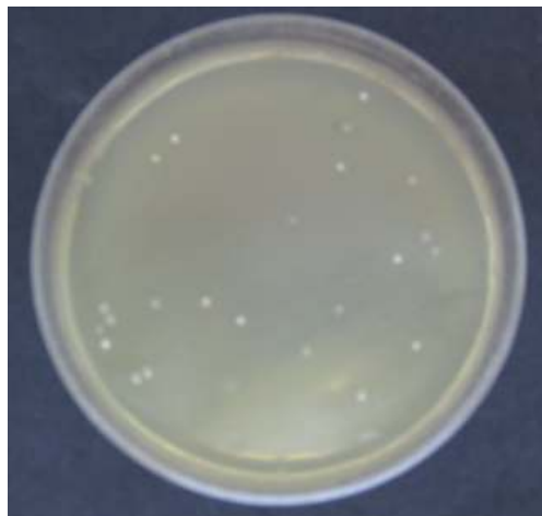
Figure 4.79 Number of S.infantis cells survived on the 1000 µg/ml silver zeolite containing plate [ 32 \pm 3 CFU/100 µl]
