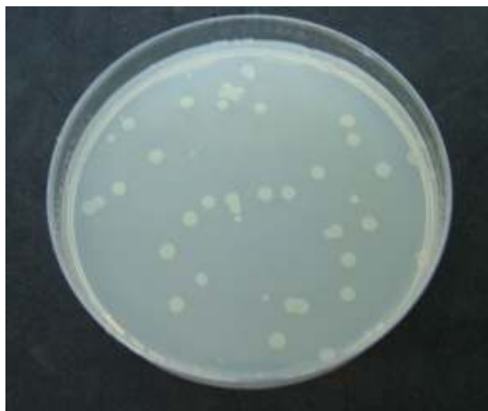
Figure 4.77 Number of E.coli cells survived on the 100 µg/ml silver zeolite containing plate [ 22 \pm 4 CFU/100 µl]
