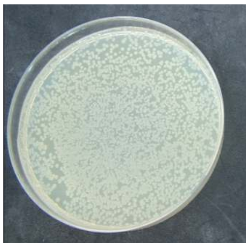
Figure 4.8 Number of E.coli cells in 100 \mu l suspension on the zeolite containing plate with 10^{-5} dilution that have 0.1 optical density value [ 740 \pm 6 CFU/100 \mu l]
