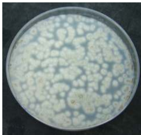
Figure 4.66 Number of A.niger cells survived on the textile that was coated with W doped \text{TiO}_2 ( 432 \pm 4 CFU/100 \mu\text{l} were counted)
