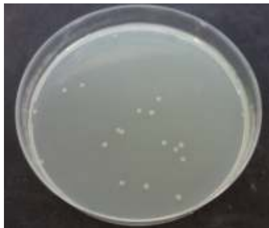
Figure 4.18 Number of E.coli cells survived on the textile that was coated with W-Zn doped \text{TiO}_2 ( 304 \pm 6 CFU/100 \mu\text{l} were counted)
