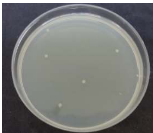
Figure 4.26 Number of S.aureus cells survived on the TiO 2 coated textile (8 ±2 CFU/100 µl were counted)
