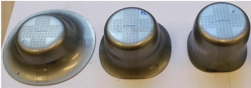
Figure 5.11 20, 35, 45 mm drawn SS304 steel cylindrical cups.
