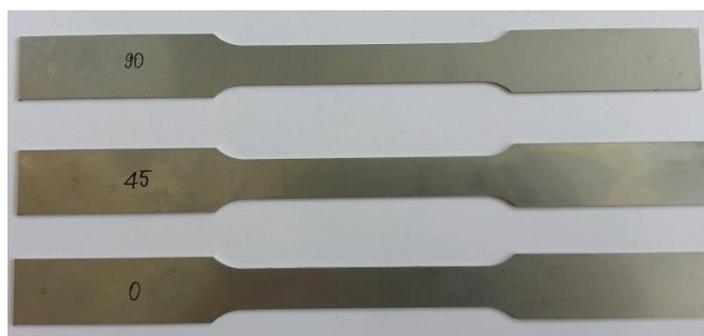
Figure 5.3 The SS304 specimens.
