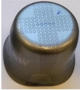
Figure 5.15 The deformed patterns on the drawn cup.
