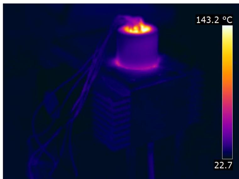
**Figure 4.17:** Thermal camera image from spraying chamber
