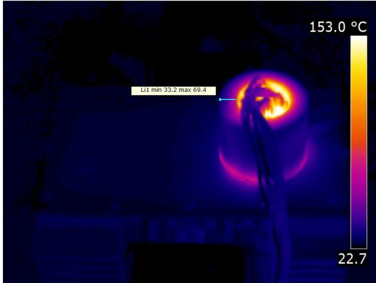
**Figure 4.18:** Cylindrical insulation jacket thermal image
