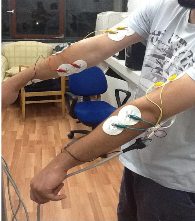
Figure 7: Electrode Placements on an Operator's Arms
