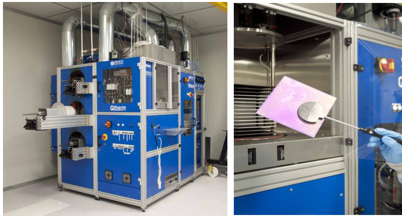
Figure 3. 34: Images of diffusion furnace and PECVD system used in GÜNAM
