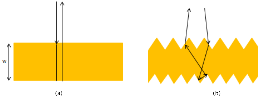
Figure 3. 6: Reflection of incident light beam from smooth surface (a), from textured surface
