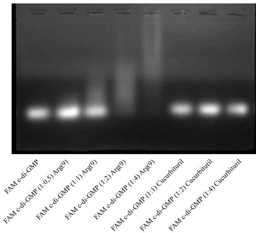
**Figure 3.2 Agarose gel electrophoresis of c-di-GMP/Arg or c-di-GMP/cucurbituril complexes.** Fluorescently labeled 2'-Fluo-AHC-c-di-GMP (0.67  $\mu$ g) was mixed with increasing molar ratios of Arg(9) (1:0.5, 1:1, 1:2 and 1:4) or cucurbituril (1:1, 1:2 and 1:4). Samples were loaded onto a 2% agarose gel and run at 70 V for 30 minutes. The bands were visualized under a UV transilluminator. The gel image is a representative of three independent experiments, each giving similar results.
