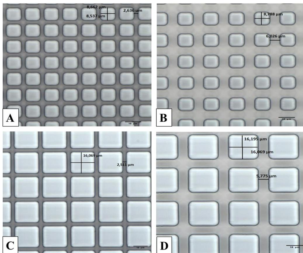
**Figure 3.3** Pillars on the silicon wafers. A)  $8.54 \times 8.66 \mu\text{m}^2$ ,  $2.64 \mu\text{m}$  gap, B)  $8.79 \times 8.79 \mu\text{m}^2$ ,  $6.07 \mu\text{m}$  gap, C)  $16.07 \times 16.07 \mu\text{m}^2$ ,  $2.51 \mu\text{m}$  gap, D)  $16.20 \times 16.07 \mu\text{m}^2$ ,  $5.78 \mu\text{m}$  gap. Pillar heights were  $6.30 \mu\text{m}$ . Micrographs were taken by light microscope. Magnification (x50). Scale bars:  $10 \mu\text{m}$ .
