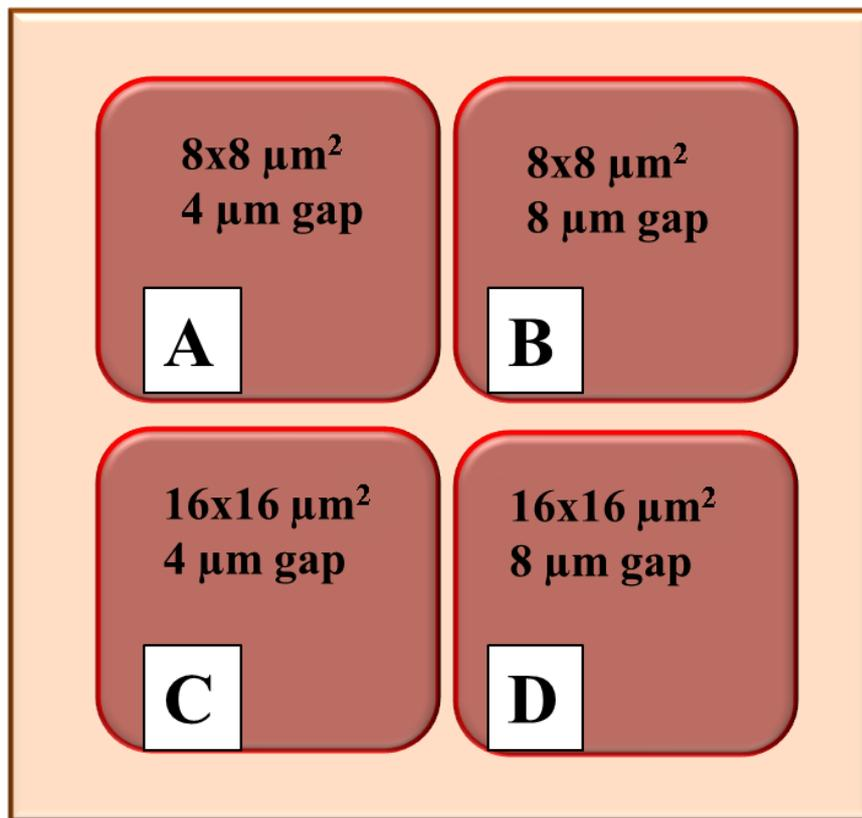
**Figure 2.1:** Image of the micropatterned silicon wafer. Silicon wafer contains 16 different patterned areas of which 4 were used in this study. Post sizes on these areas were designed to have dimensions of 8x8 μm<sup>2</sup> and 16x16 μm<sup>2</sup> with spacings of 4 μm and 8 μm and post height of 5 μm. A) 8x8 μm<sup>2</sup>, gap 4 μm, B) 8x8 μm<sup>2</sup>, gap 8 μm, C) 16x16 μm<sup>2</sup>, gap 4 μm, D) 16x16 μm<sup>2</sup>, gap 8 μm.
