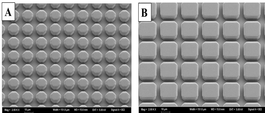
**Figure 3.2** SEM micrographs of the main template with  $5 \mu\text{m}$  micropillar height. Tilt angle of the stab:  $31.6^\circ$ . A)  $8 \times 8 \mu\text{m}^2$ , gap  $8 \mu\text{m}$ , B)  $16 \times 16 \mu\text{m}^2$ , gap  $8 \mu\text{m}$ . Magnification (x2000).
