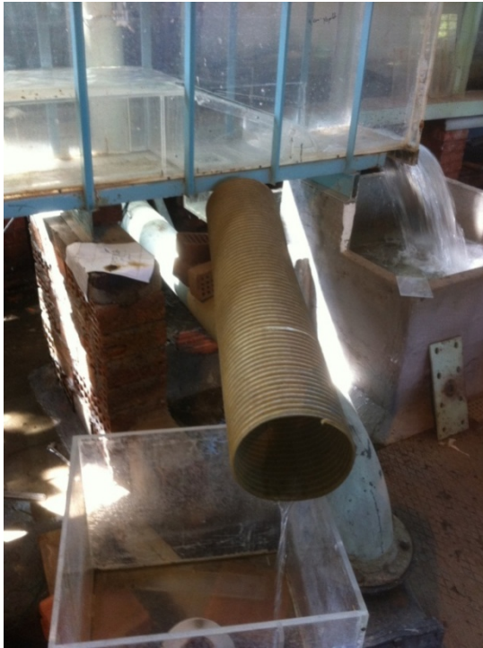
Figure 3.8: General view of the tank in which water coming from the orifices is collected
