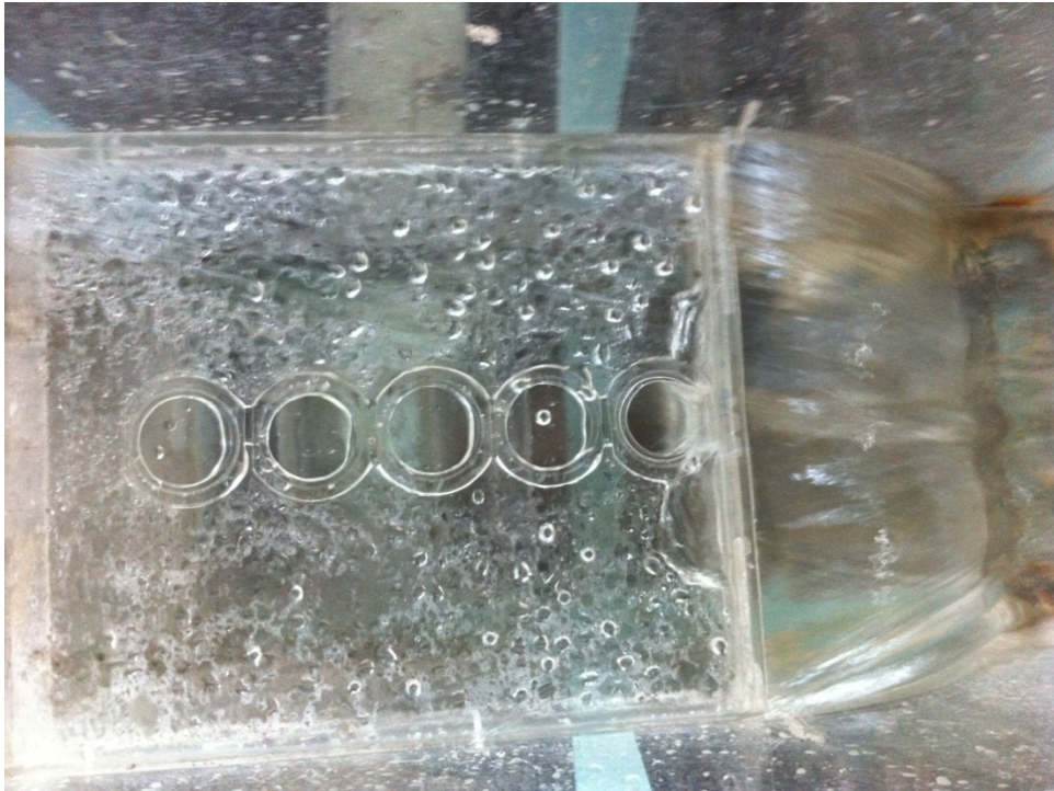
Figure 3.4: Top view of the circular bottom intake orifices
