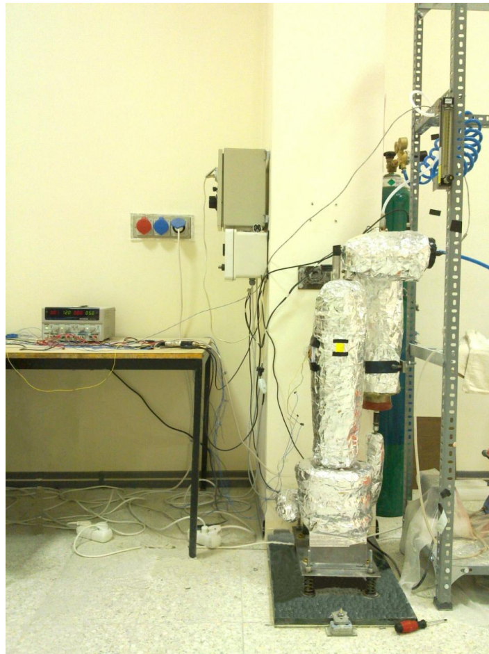
Figure 3.8 A photograph of the vibrated fluidized bed dryer system
