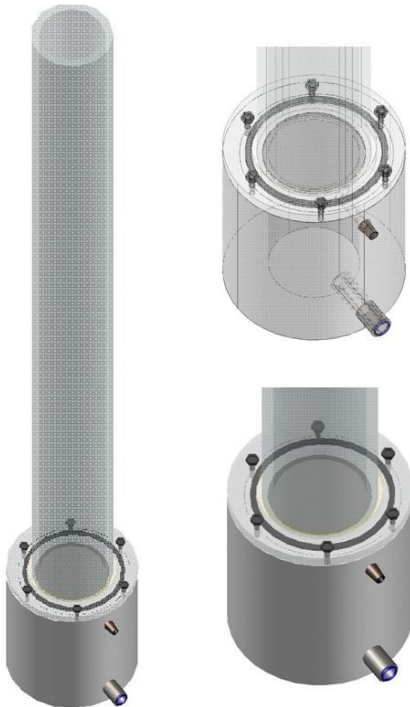
Figure 3.2 Fluidized bed apparatus used in hydrodynamic experiments
