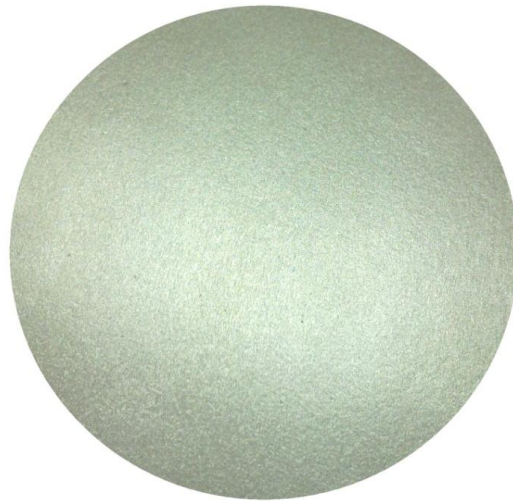
Figure 3.4 Sintered porous metal gas distributor
