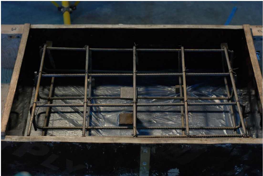
Figure 1.14 Push-Out Specimen with Reinforcement
