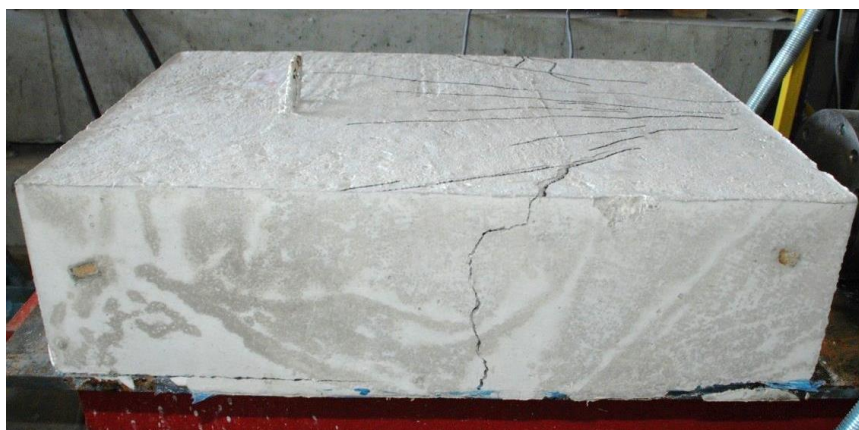
Figure 1.20 Surface Cracking – U140 x 75mm
