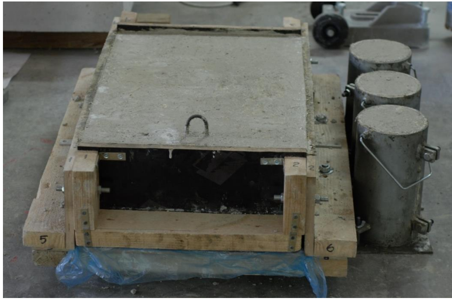
Figure 1.13 Push-Out Specimen and Cylinders
