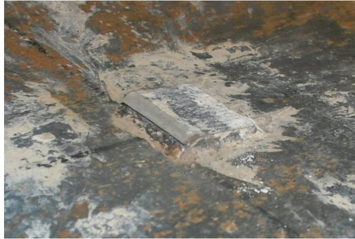
Figure 1.16 Chanel Fracture – Base Plate
