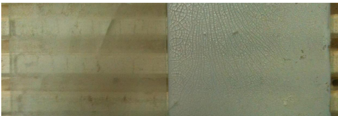
Figure 15. Picture of glasses coated by sol-gel method (on the left side) and doctor blade method (on the right side)
