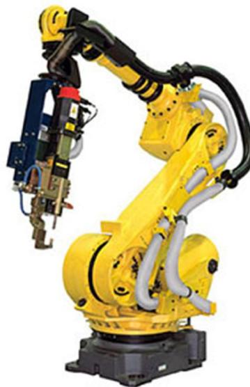
Figure 1 - An example of industrial robots; welding robot [1].
