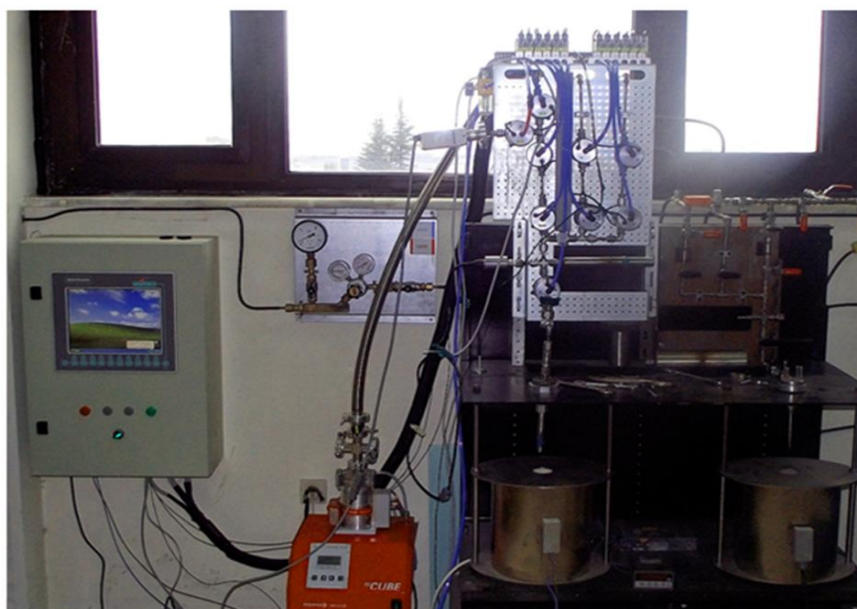
Figure 3.4 Custom-made apparatus used for decrepitation treatment.
