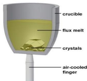
Figure 2.9 Schematic representation of Flux melting technique [46]
