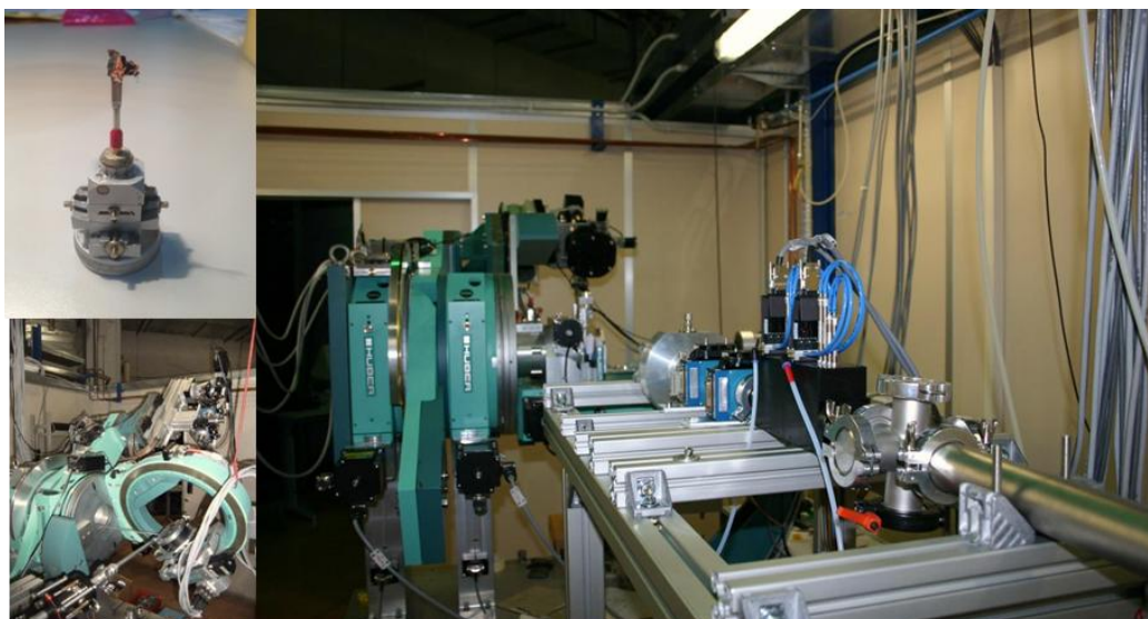
Figure 2.10 Flat sample holder and MCX beamline experimental hutch.
