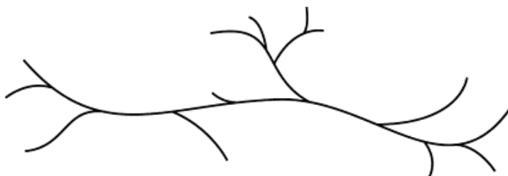
Figure 1.1 Chain configuration of LDPE
