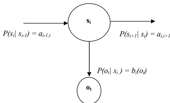
**Figure 8** The Representation of an HMM
