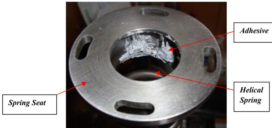
**Figure 4.3.** Application of Elastic Adhesive Between Seat and Spring
