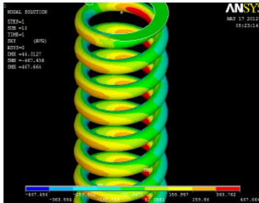
**Figure 2.23.** Shear Stress Distribution [13]
