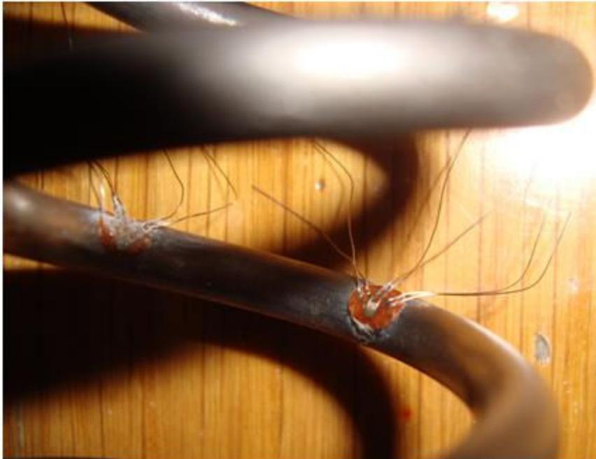
**Figure 4.5.** Strain Gage Close View
