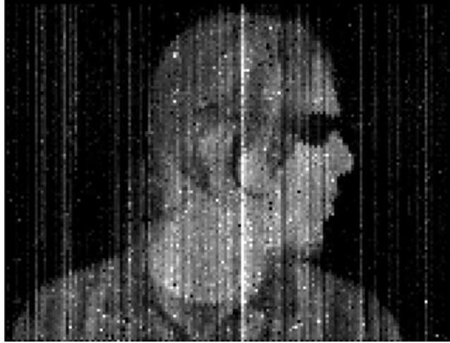
Figure 1-5: The first successful room temperature image taken with the diode type microbolometer at METU with SOI-CMOS diode microbolometer array with a pixel pitch of 70 \mu\text{m} designed in 2011 [21].
