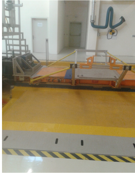
Figure 106 The dummy weights used during the iteration of the parameters of the electronic control unit of the sled's accelerator for each pulse severity
