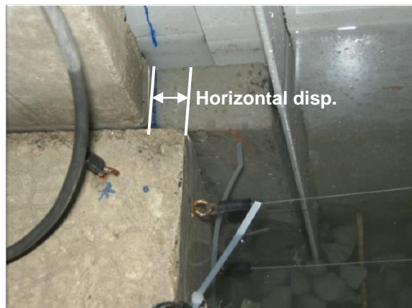
Figure 7.22: Horizontal displacement measurement for two blocks (Block 2) for Soil 1
