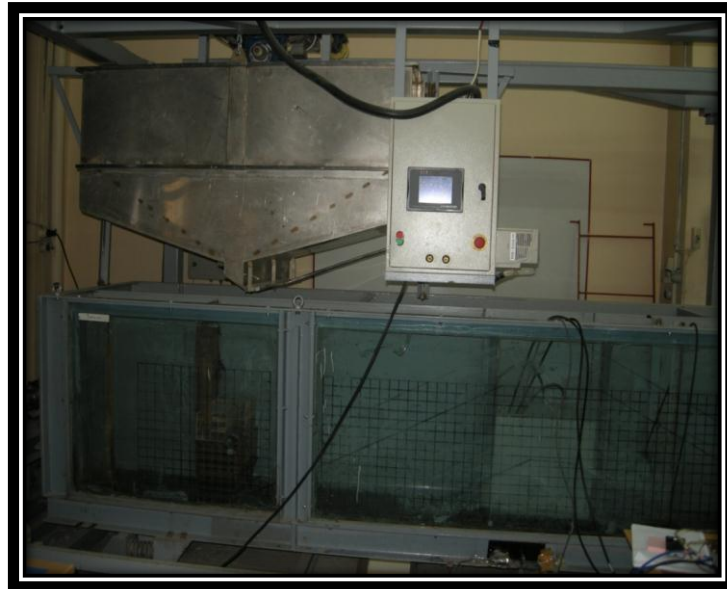
Figure 4.5: Raining system and shaking table
