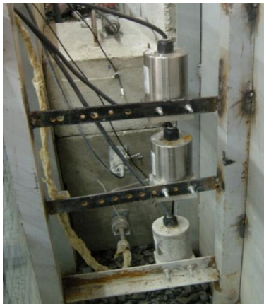
Figure 7.33: Placements of the position transducers (P1, P2, P3) for three block tests for Soil 1
