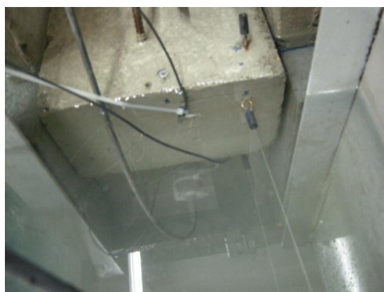
Figure 7.24: Position of the Block 2 after dynamic loading (after 5 Hz)
