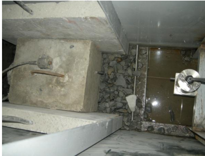
Figure 7.13: Position transducer for one block test for Soil 2
