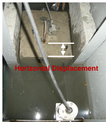
Figure 7.8: Position transducers for one block tests for Soil 1
