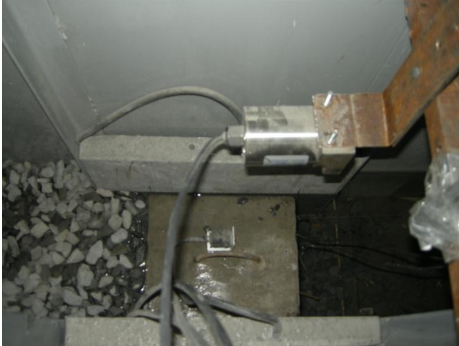
Figure 7.2: Position transducers for one block tests for Soil 1
