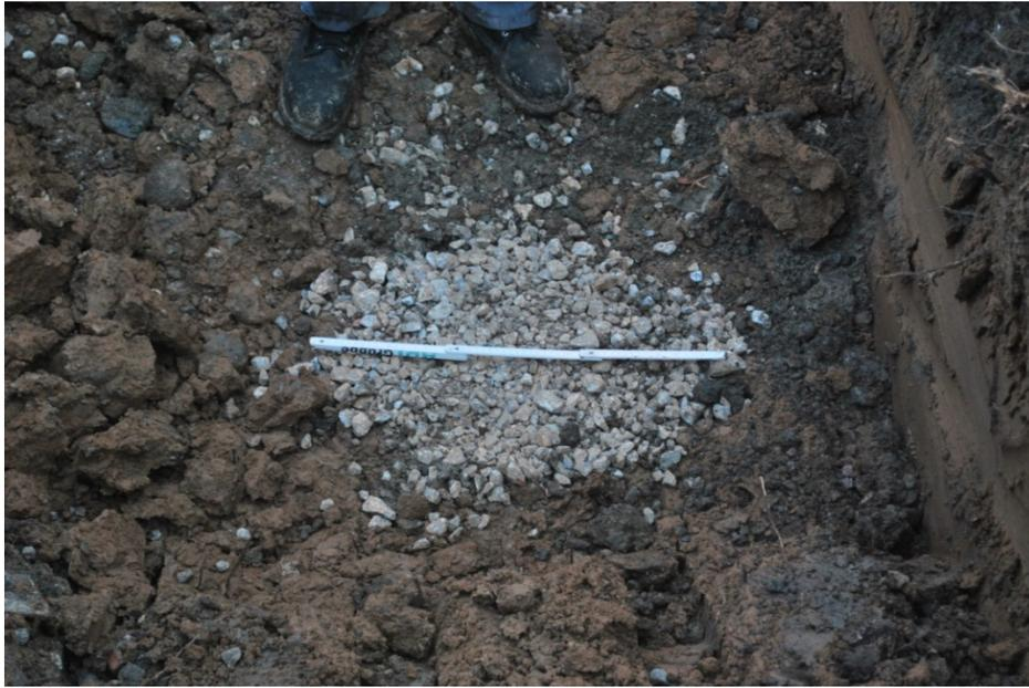
Diameter measurement of a constructed rammed stone column
