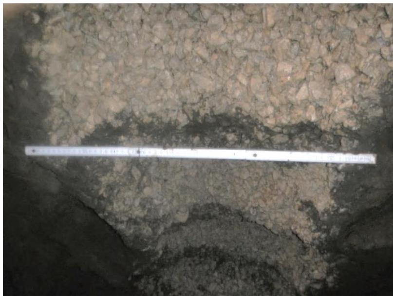
Appearance of the constructed rammed stone column after excavation of the surrounding soil
