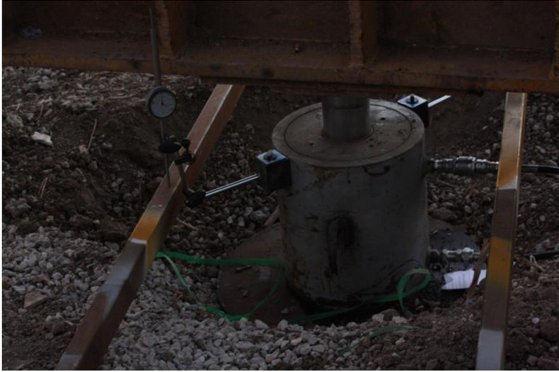
A view of the load test on a single rammed stone column
