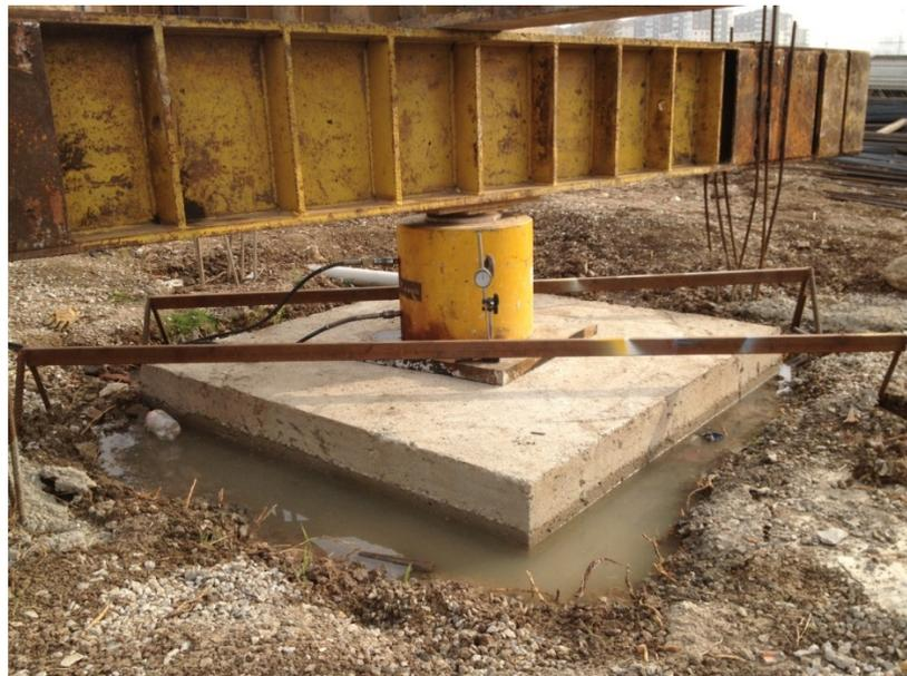
A view of the load test on a group of rammed stone columns
