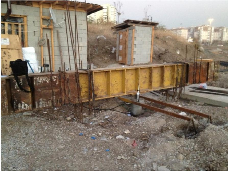
Figure 3.5 Set up of the single rammed stone column test
