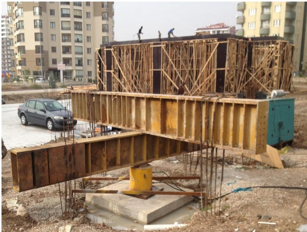
Figure 3.7 A view of the group load test setup
