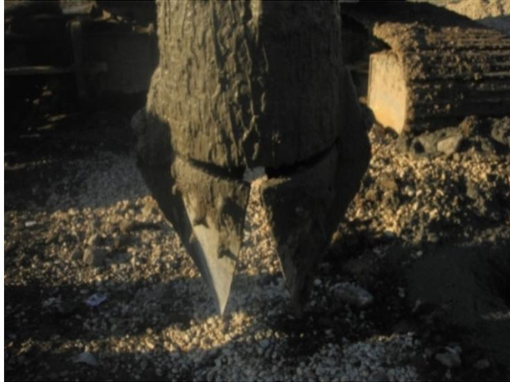
Figure 3.3 Tamper at the tip of the drill rig
